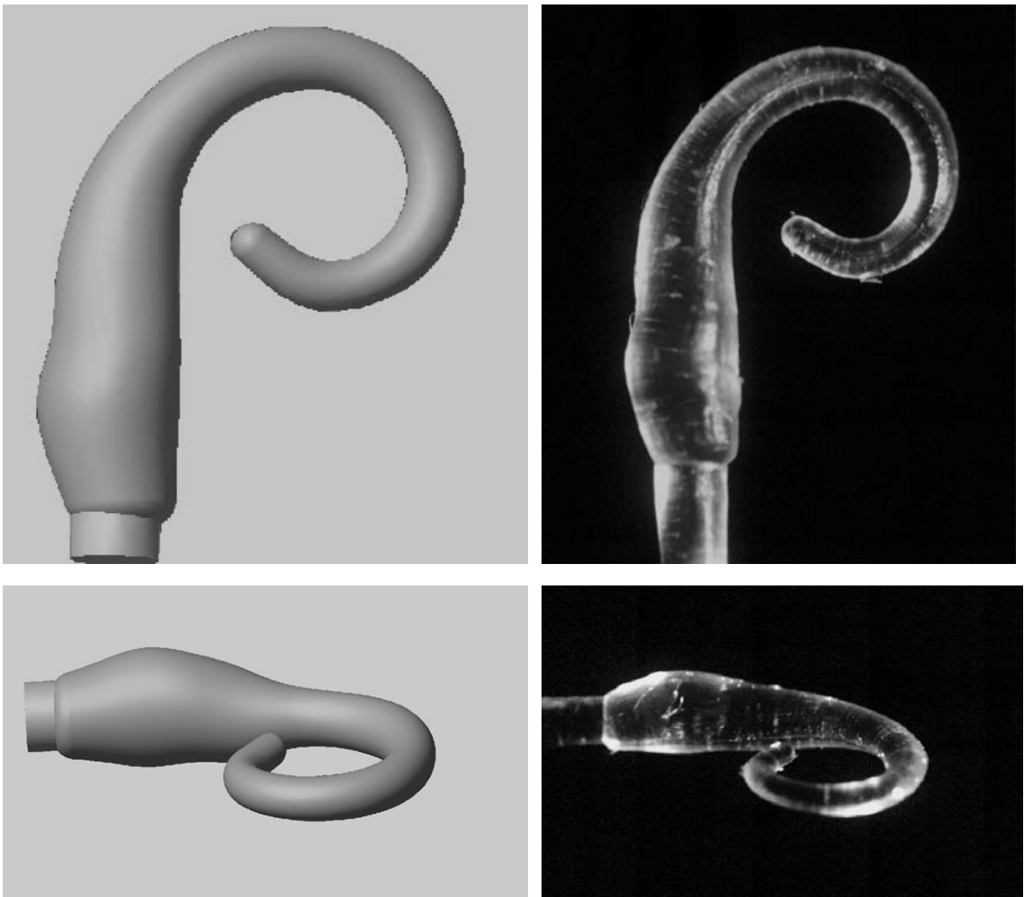
Figure 3. Rendered CAD images (left) and silicone molded parts (right).
