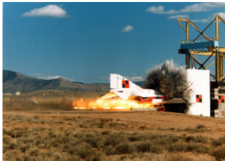
CRASH TEST: Among the more dramatic tests to be conducted at Sandia's rocket sled track facility is this crash of a complete F-4 Phantom into a massive reinforced concrete target to estimate the effect of a crash into a nuclear power plant containment building.
