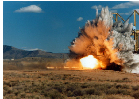
CRASH TEST: Among the more dramatic tests to be conducted at Sandia's rocket sled track facility is this crash of a complete F-4 Phantom into a massive reinforced concrete target to estimate the effect of a crash into a nuclear power plant containment building.
