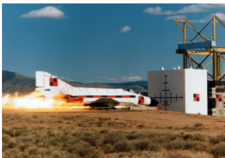
CRASH TEST: Among the more dramatic tests to be conducted at Sandia's rocket sled track facility is this crash of a complete F-4 Phantom into a massive reinforced concrete target to estimate the effect of a crash into a nuclear power plant containment building.
