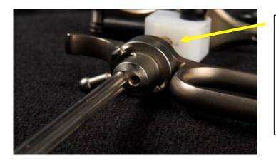
A hole within a Teflon block that is part of the resectoscope system's working element. While not obvious to the user, this hole comes into play when determining the reprocessing for this device.
