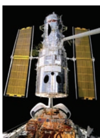
Attached to the "robot arm," the Hubble Space Telescope is unberthed and lifted up into the sunlight during the telescope's second servicing mission.
