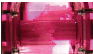
The heart of the Bioreactor Demonstration System (BDMS) is the rotating wall vessel, shown here without its support equipment. During the mission, astronauts studied the interaction of prostate cancer cells and bone cells by using a BDMS to form large samples for research.
