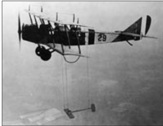
Airfoil research took many different forms. At NACA's Langley Memorial Aeronautical Laboratory in 1921, the performance of a model wing was tested by being suspended beneath a Curtiss JN-4 "Jenny" aircraft, which employed a Royal Air Force 15-airfoil section. NASA Image #L-00130 (LaRC)
