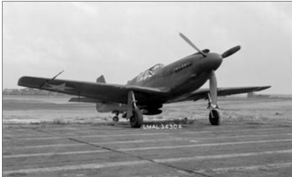
One of the reasons why many experts feel the North American P-51 Mustang represents the highest level of technical achievement ever accomplished in a propeller-driven fighter aircraft is its highly effective low-drag wing. The XP-51 was the first aircraft to incorporate a NACA laminar-flow airfoil. This is the second XP-51, which arrived at Langley in March 1943. NASA Image #L-34304 (LaRC)
