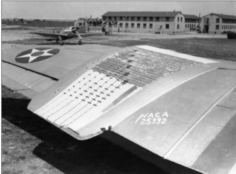
In the spring of 1941, NACA Langley installed an experimental low-drag test panel on the wing of a Douglas B-18 airplane. The panel was fitted with suction slots and pressure tubes for a free flight investigation of the transition from laminar to turbulent flow in the boundary layer. Liquid manometers installed in the fuselage measured the pressure at each tube. NASA Image #L-25332 (LaRC)
