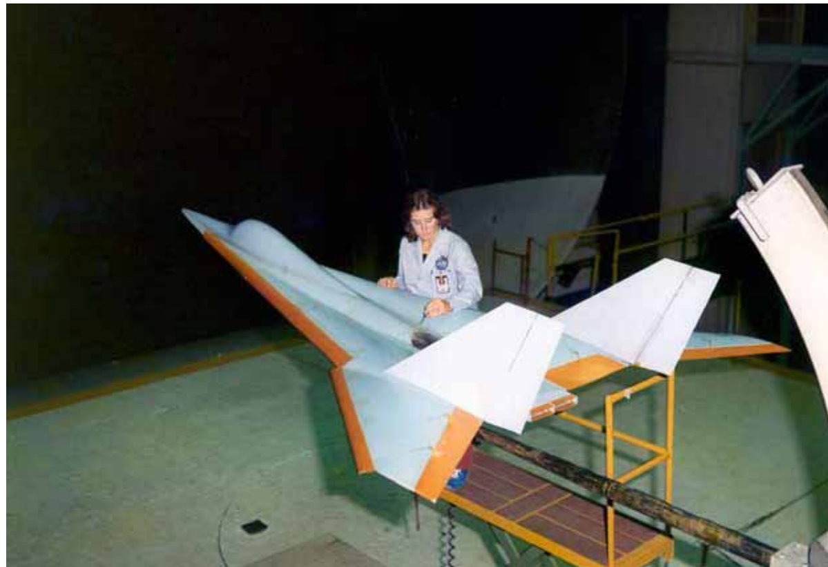
Model of a Langley-designed supersonic-cruise fighter concept (SCIF-IV) in the Langley Full-Scale Tunnel in 1977.
