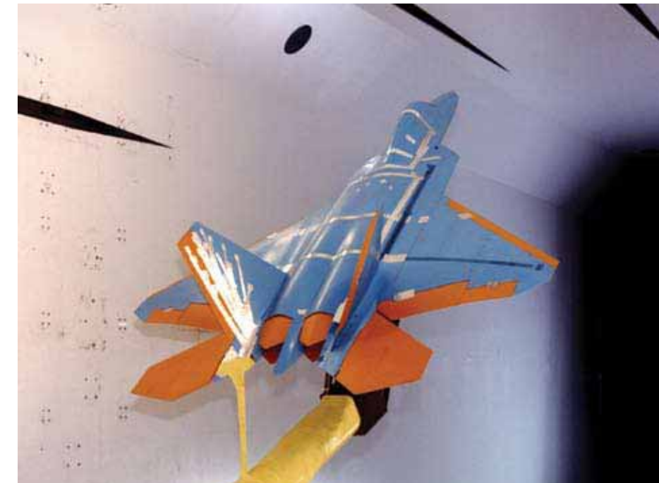
F-22 model mounted in Transonic Dynamics Tunnel for tail buffet studies.
