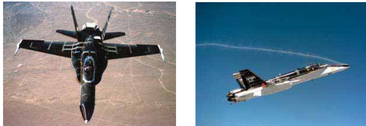
In-flight pictures of the High Angle-of-Attack Research Vehicle showing the right strake deployed (left) and smoke-flow visualization of the vortex path shed by the strake (right)
