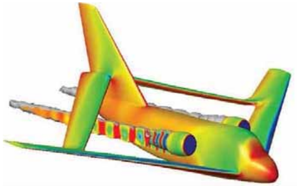
Computational simulation of power-induced flow on the RevCon Joined-Wing Flight Demonstrator.
