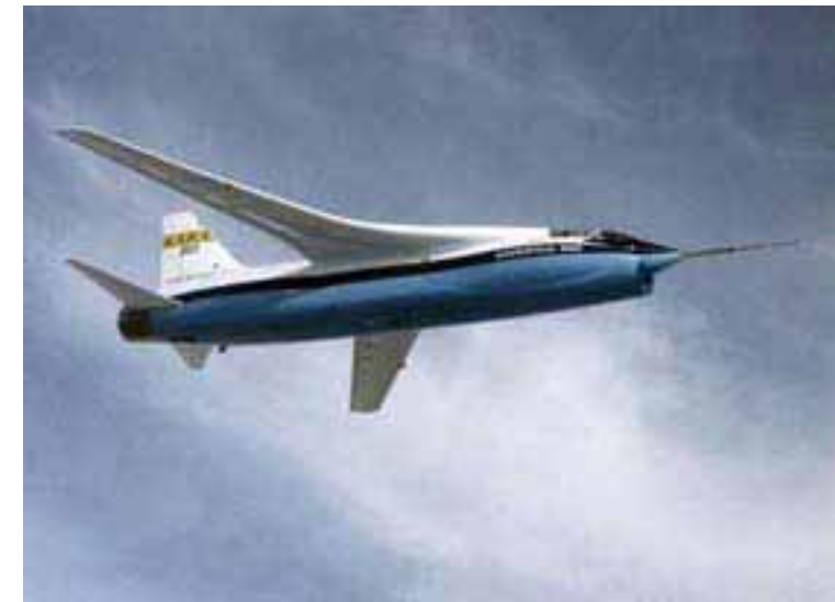
NASA F-8 research airplane with supercritical wing used as basis for design of ARW-1 wing.
