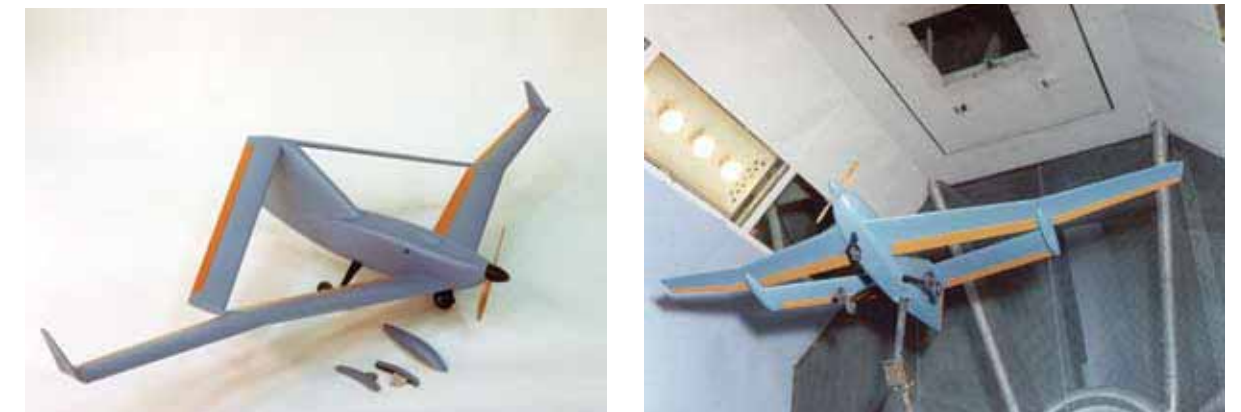
Advanced agricultural airplane model tested at Langley.
