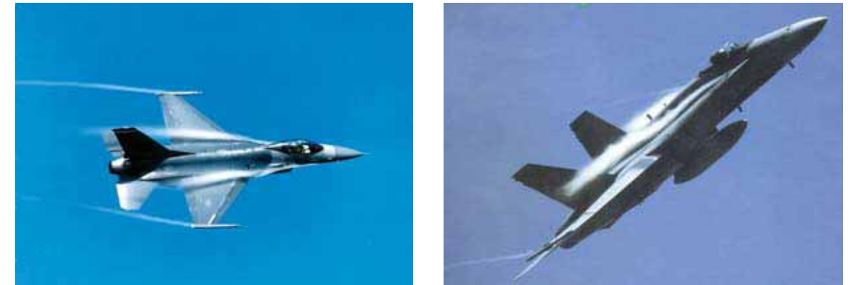
The F-16 (left) and the F/A-18 (right) use vortex lift for improved maneuverability.
