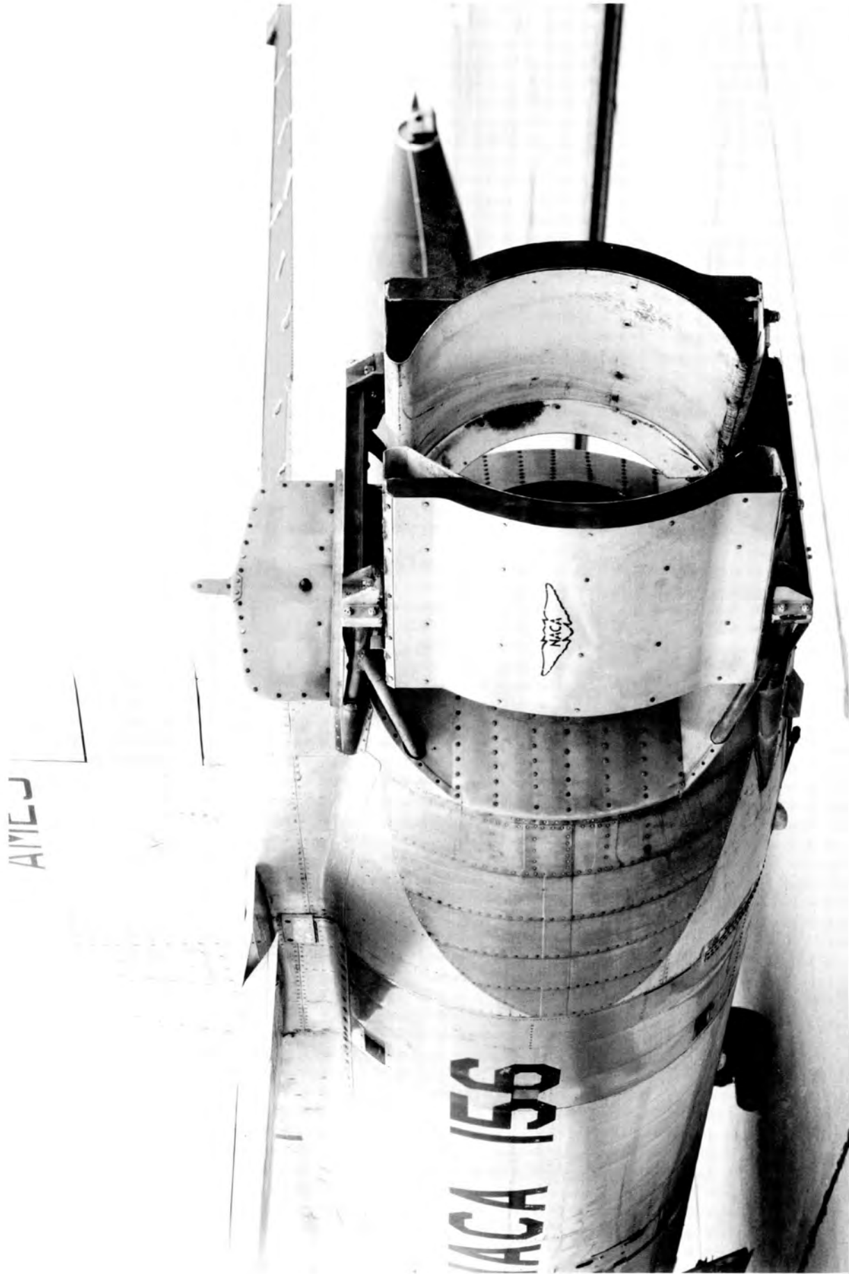
Figure 62. Close-up of target-type thrust reverser in forward thrust position (on F-94C Starfire). Titanium skin was added on the rear fuselage to withstand high-temperature environment. (1958) A-24153-2A
