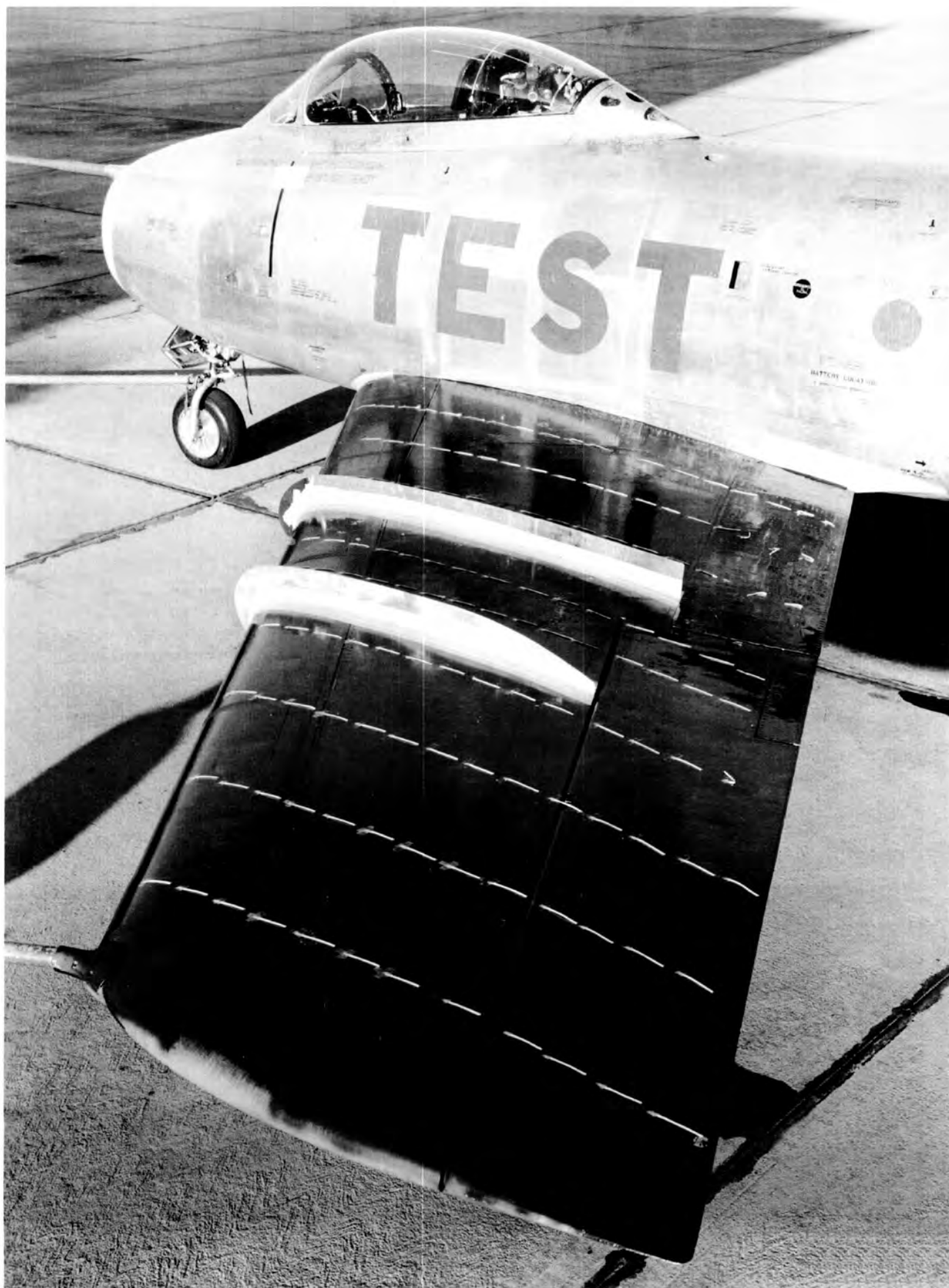
Figure 51. Multiple fences on F-86A wing reduced flow separation outboard with less roll-off at stall. Additional fences strongly reduced wing maximum lift. (Nov. 1952) A-17733
