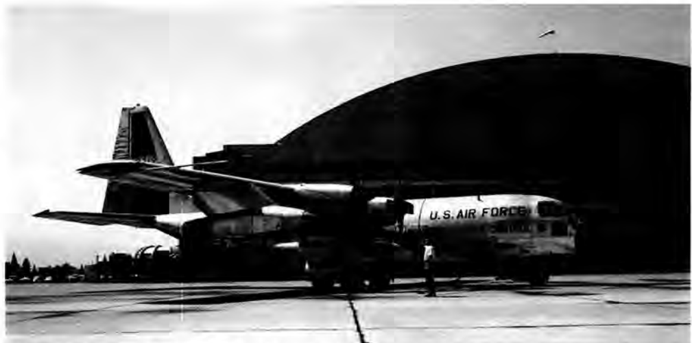
The Lockheed NC-130B STOL turboprop-powered aircraft in front of the NASA hangar (Sept. 1961).
