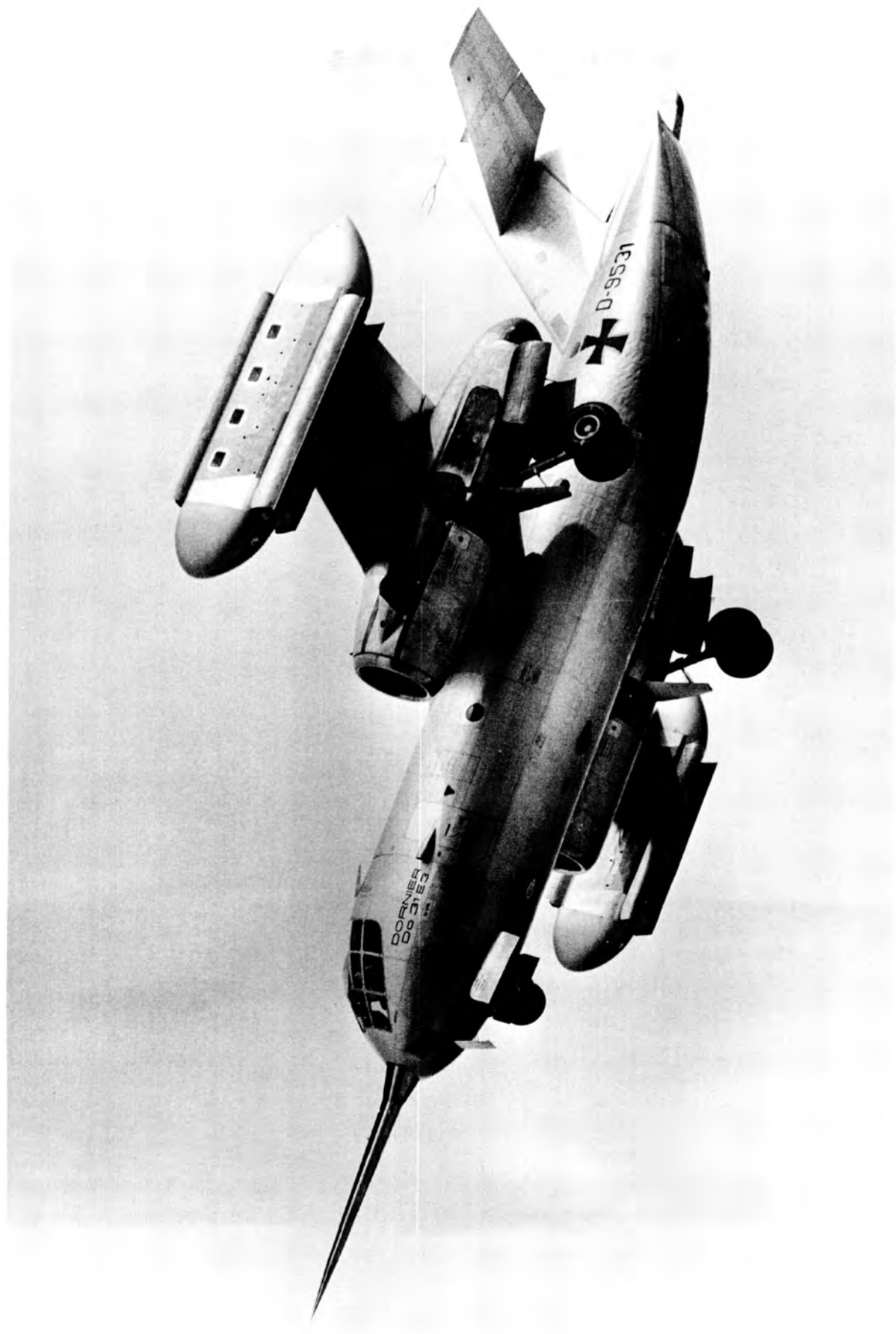
Figure 105. The Dornier DO-31, an experimental V/STOL transport, in forward flight. Four turbojet lift engines were mounted in each of two removable wing pods; they were modulated for roll control in hover and low-speed flight. Two vectored-thrust Pegasus main engines (15,000 pounds thrust each) provided Mach 0.6 cruise speed. (Dec. 1969) A-42712-2
