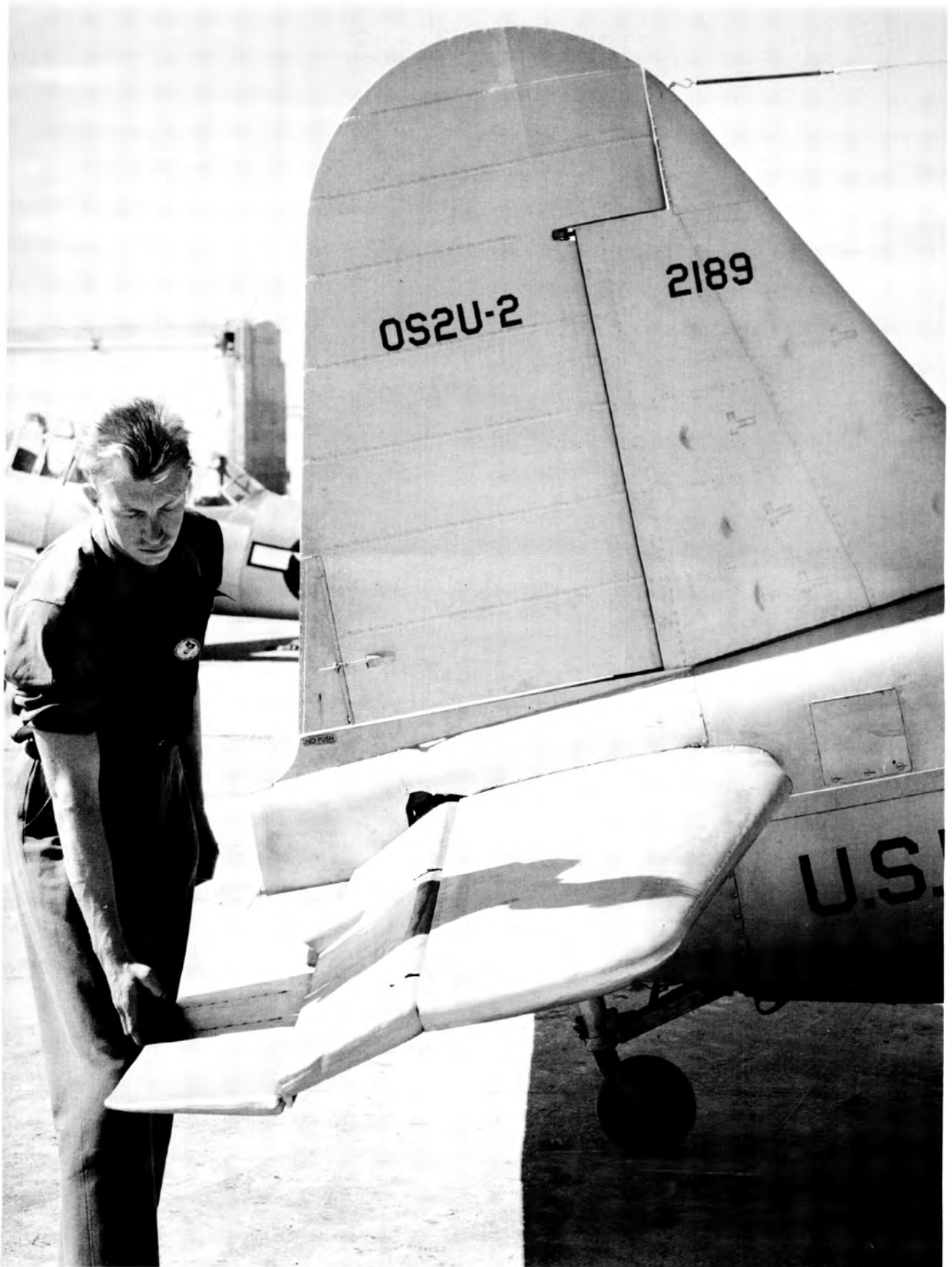
Figure 56. Ames-designed, double-hinged horizontal tail mounted on the OS2U-2 Kingfisher provided increased lift for maneuvering and landing (Vultee BT-13 in background). (Feb. 1945) A-7431
