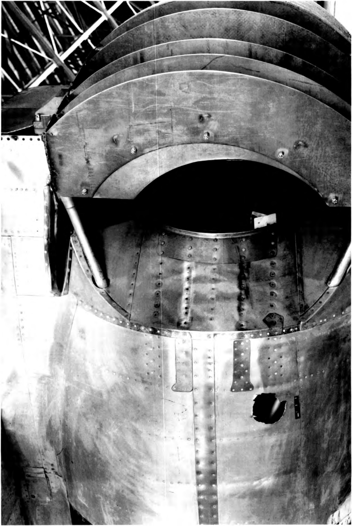
Figure 61. Close-up of damage to rear fuselage of F-94C Starfire caused by hot engine exhaust gases during prolonged use of thrust reverser in landing rollout. Fairing to cover rear portion of reverser has yet to be added. (Sept. 1957) A-23157
