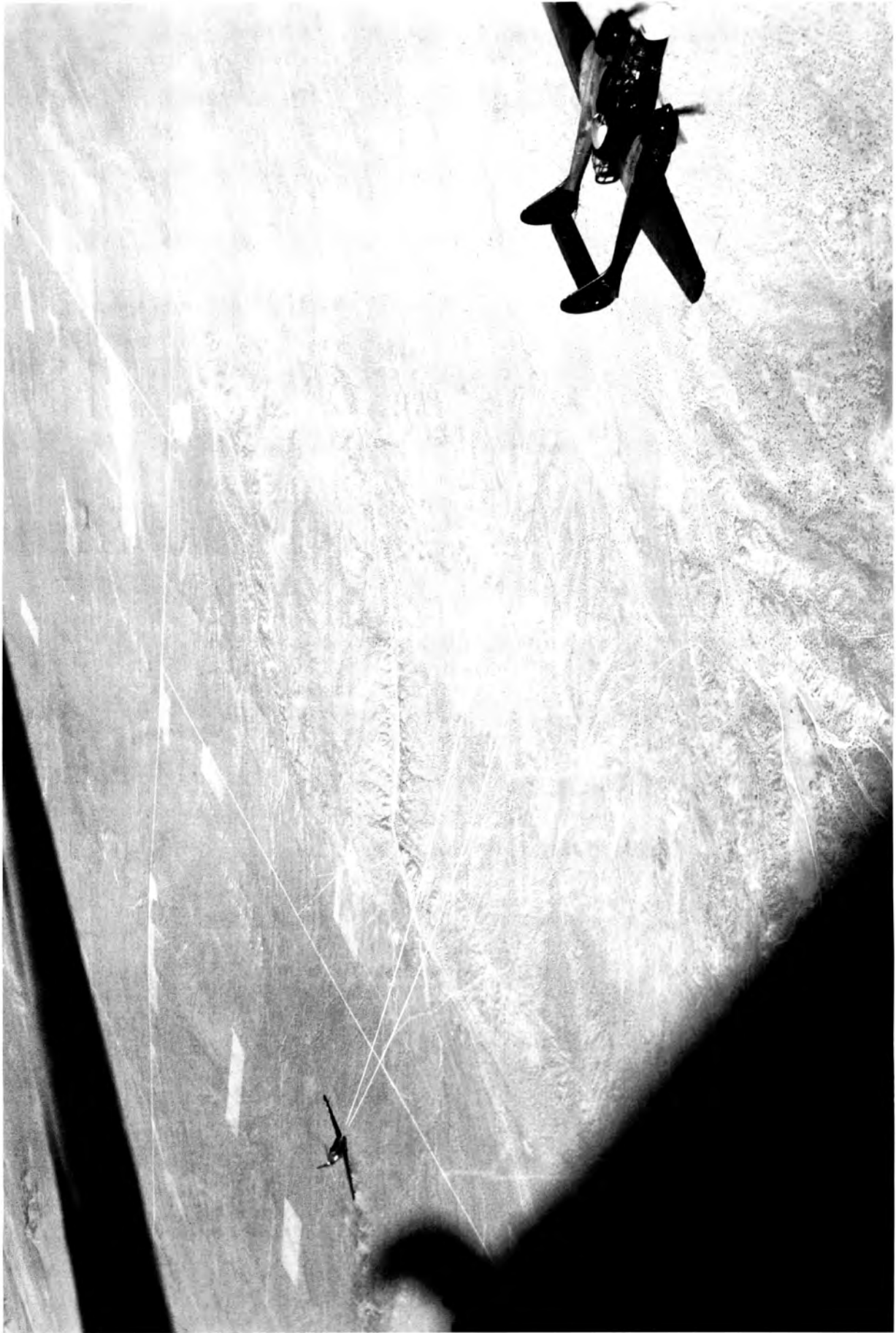
Figure 24. North American P-51B towed to an altitude of 28,000 feet by a Northrop P-61 Black Widow over Muroc Dry Lake, California. After the pilot released the tow cable, drag measurements were obtained at various airspeeds in a 20-minute unpowered flight. (Sept. 1944) A-6538
