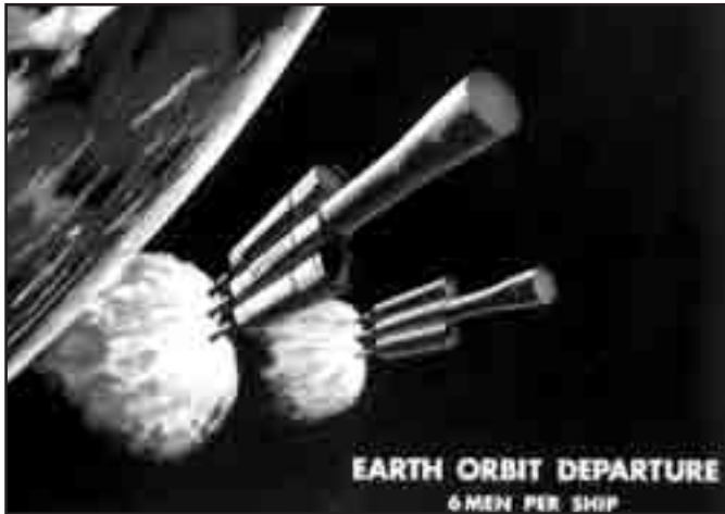
Figure 15—Twin Mars ships blast their all-male crews from Earth orbit using NERVA nuclear rocket stages. In August 1969, Wernher von Braun used images such as this to present NASA's vision of a Mars expedition in the 1980s to the Space Task Group and to Congress. (NASA Photo MSFC-69-PD-SA-176)
