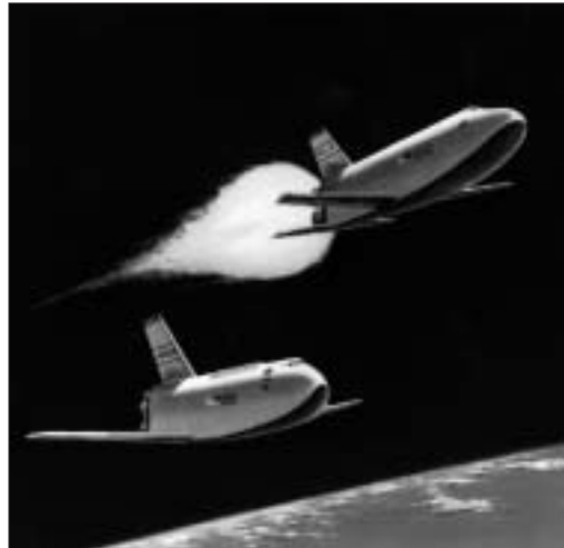
Figure 2-2. This artist's conception, also from 1969, shows a fully reusable Space Shuttle at the point of separation when the orbiter leaves the atmosphere. The larger vehicle that boosted the orbiter was then to be piloted back to Earth. (NASA photo)
