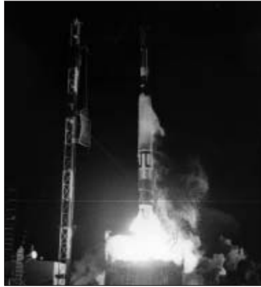
Figure 1-3. A test of the Viking rocket used to launch the Vanguard satellite, TV 3 BU. This satellite was part of the U.S. Earth satellite program to place in Earth orbit the first American satellite on February 5, 1958. The satellite would measure atmospheric density and conduct geodetic measurements. After 57 seconds of flight, connection units of the first-stage control system failed. At 20,000 feet, the rocket veered off course and broke apart. Not until March 1958 did Vanguard I successfully enter Earth orbit. (NASA photo VAN 9A)
