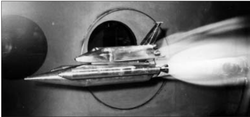
Figure 2-4. Ames Research Center scientists tested the aerodynamic properties of a Space Shuttle wind tunnel model in 1973. (NASA photo)
