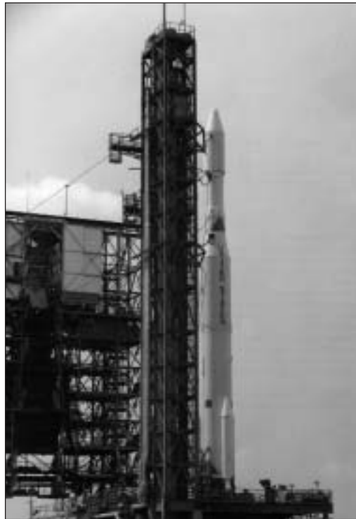
Figure 1-4. This photograph of a long-tank Delta no. 73 rocket was taken on August 22, 1969, at Kennedy Space Center in Florida. It shows the launch configuration for the Pioneer E, which would have been called Pioneer 10. When launched on August 27, however, the launch vehicle malfunctioned and was destroyed 8 minutes and 3 seconds into powered flight by the range safety officer. (NASA photo 69-H-1442)
