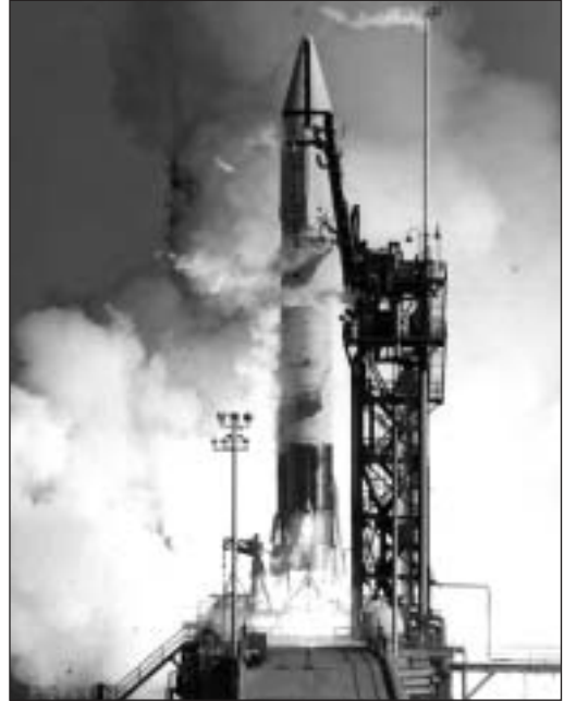
Figure 3-4. The Atlas-Centaur two-stage rocket has been a reliable launcher for the United States since the 1960s. Here an Atlas-Centaur carries a test article for the Surveyor spacecraft program into space on December 11, 1964. (NASA photo 64-H-2808)
