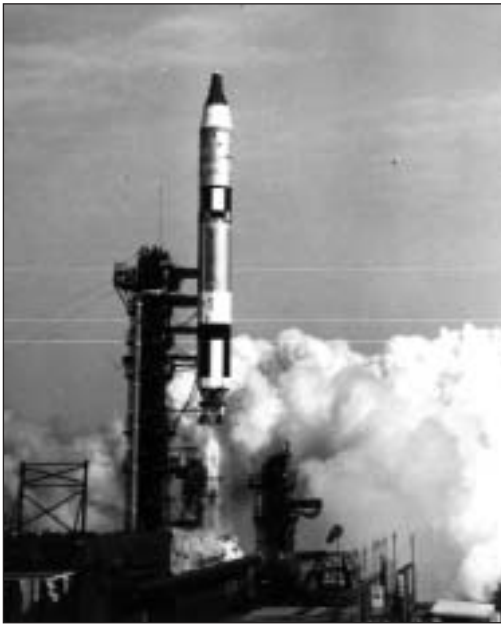
Figure 1–7. The launch of the first piloted mission of the Gemini program, Gemini 3, atop the sturdy and reliable Titan launch vehicle. The Titan was originally developed as part of the Air Force’s ICBM program in the late 1950s. This launch took place on March 23, 1965, with astronauts Gus Grissom and John Young aboard. (NASA photo 65-H-448)
