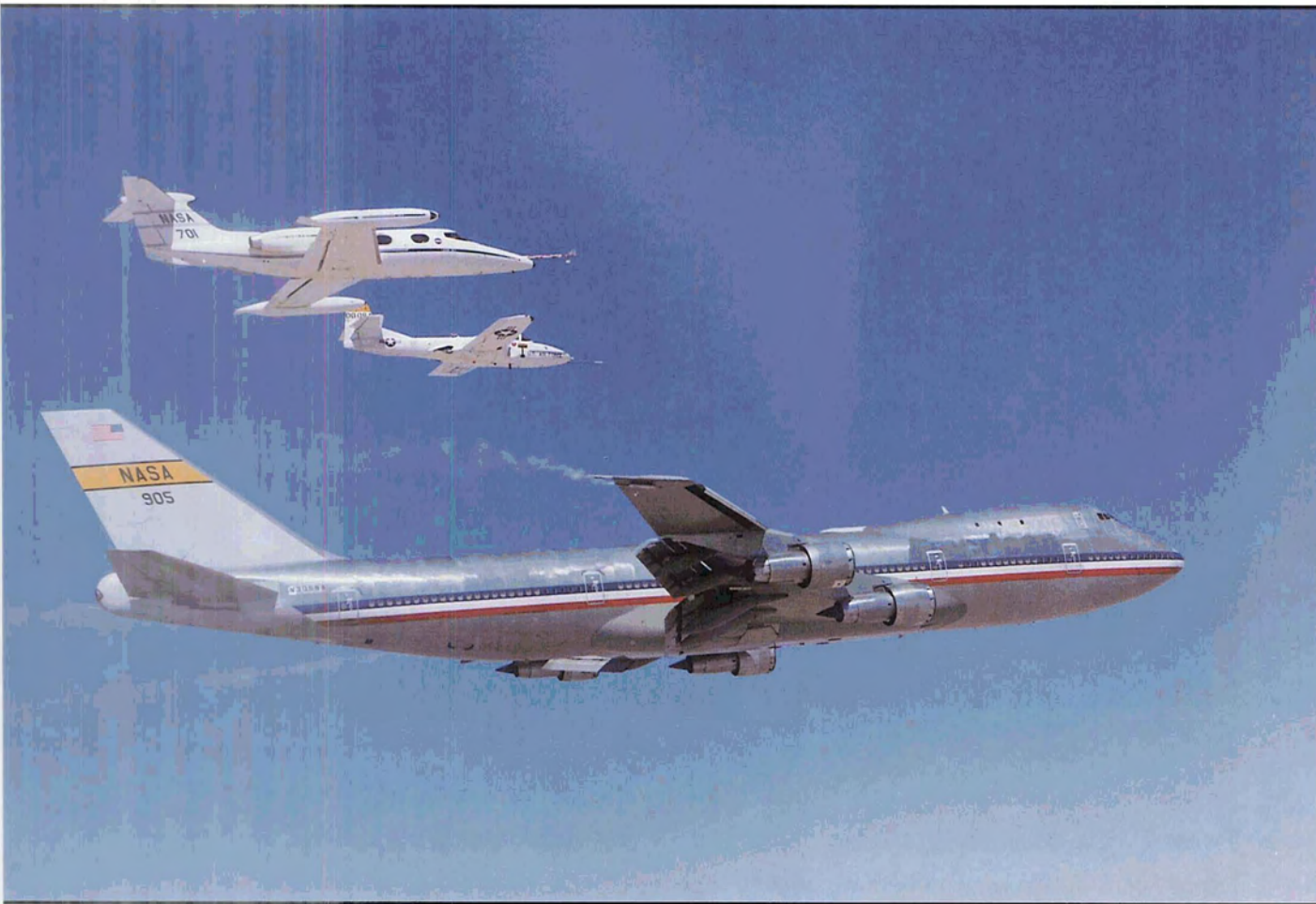
747 wake vortex research with smoke generators. A Learjet and T-37 Cessna are flying through the wake to measure the forces and effects of the vortices. (NASA Photo ECN 4243)
