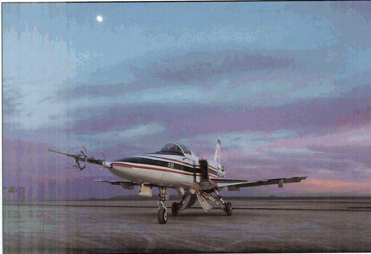
X-29s on lakebed near sunrise with the Moon still visible. (Pitot tube of second aircraft at viewer's left.) Both of these forward-swept-wing aircraft were flown at Dryden from 1984 to 1992 as technology demonstrators to investigate a host of advanced concepts and technologies. These included advanced composite materials, the forward-swept wing, and a computerized fly-by-wire flight control system that overcame the aircraft's inherent instability. The 434 total missions flown by the two X-29s provided an engineering data base that is available in the design and development of future aircraft. (NASA Photo EC90 357-7)
