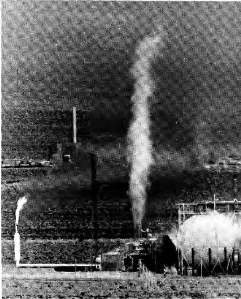
December 15: The Nuclear Rocket Development Station at Jackass Flats, Nevada, as the NERVA nuclear rocket reactor, NRX-A6, is operated at or above design power of 1,100 mw energy (55,000-lb thrust) for 60 min.
