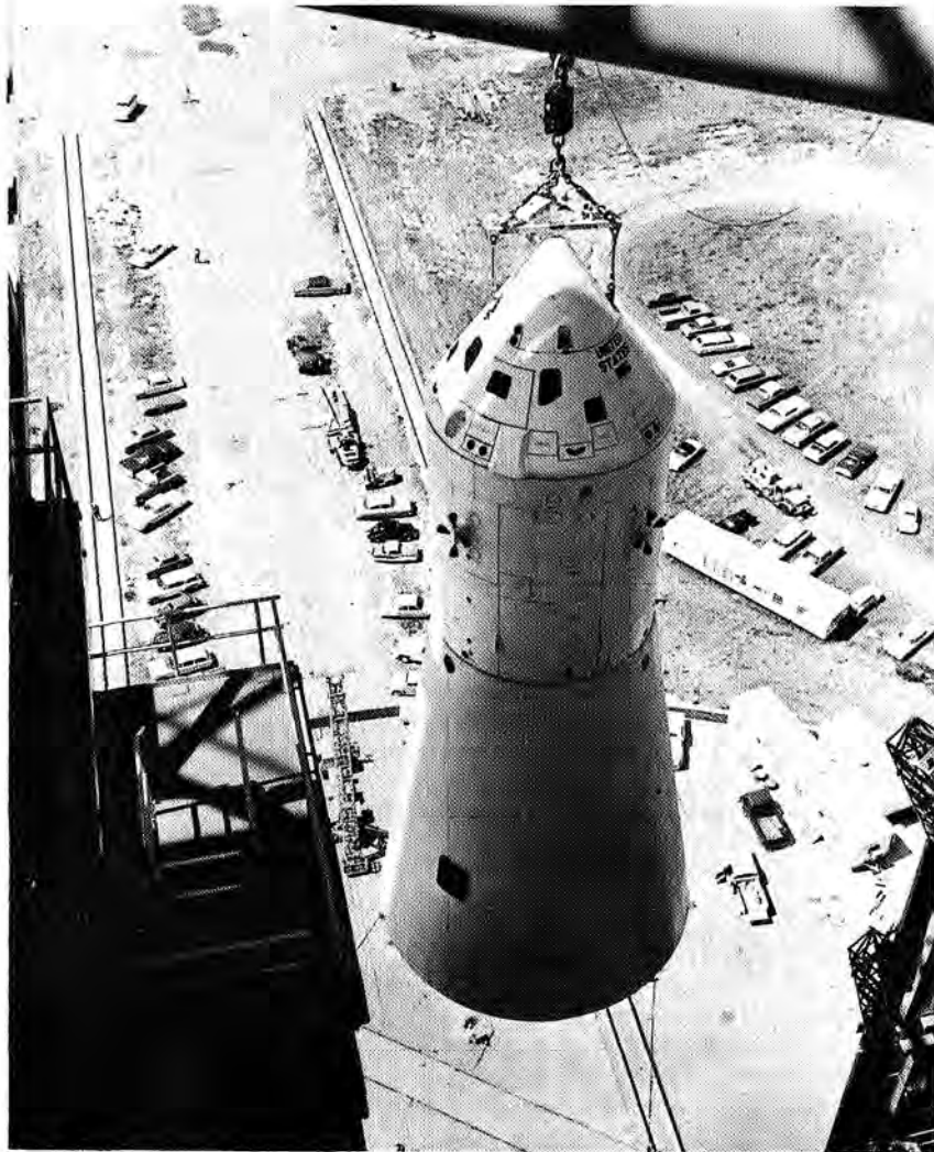
January 4: Apollo spacecraft—command module, service module, and adapter section—is raised up the gantry for mating to Saturn IB launch vehicle at Launch Complex 34, Eastern Test Range.
