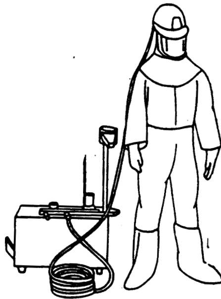
A sandblasting hood (a respirator)
