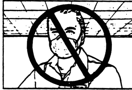
A dust mask is not a respirator
