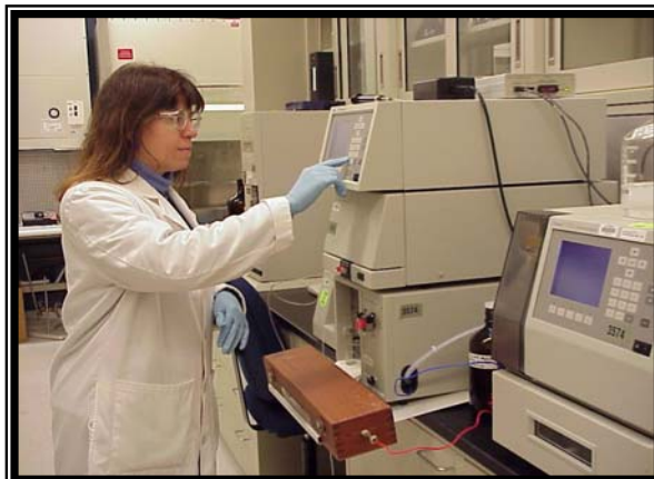
Chemist Beth Brown performs a dose certification HPLC analysis in support of an FDA-nominated NTP study.
