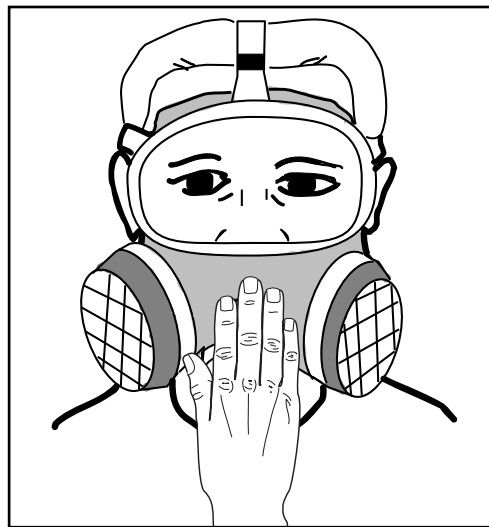
Figure 5-9. Cover the exhalation valve when performing a positive pressure user seal check
