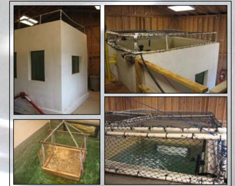
One of two dive tanks (2.4 m x 1.8 m x 2.4 m) used for diving energetics studies with ducks at Patuxent Wildlife Research Center
