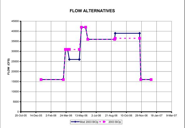
Figure 2 Fall back plan for Gavins Point flow releases as per the 2003 amended biological opinion and including the summer-flow exemption. Plan assumes 'normal flow' conditions and is termed '2003 BiOp'. A modification of '2003 BiOp' termed Mod 2003 BiOp is also shown.
