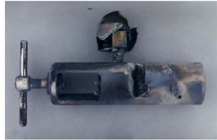
Fig. 3 Remains of exploded regulator after test
