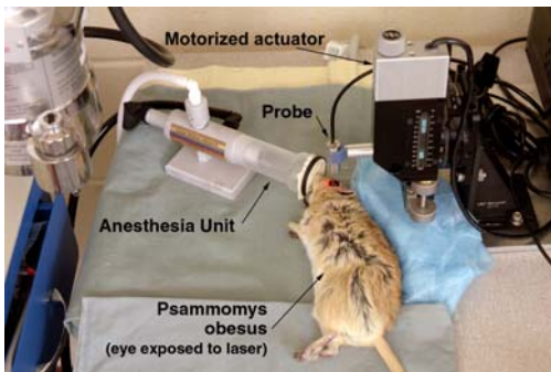
Fig. 4c. Close-up view of experimental set-up for prototype dynamic light scattering ocular probe, sand rat and anesthesia unit.
