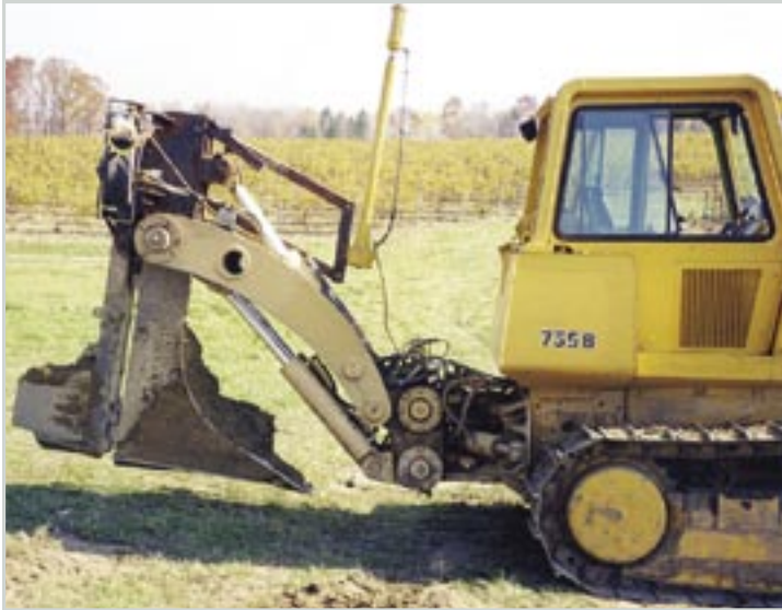
FIGURE 8. Equipment used to install drain tile between rows in a vineyard with imperfect soil drainage. Photos courtesy of Gene Sigel.
