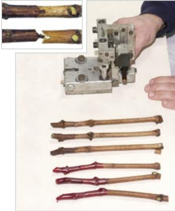
FIGURE 19. Bench grafting: Grafting machine with grafted and waxed cuttings. Insert: Omega cut graft. Scion (left); disbudded rootstock (right).
