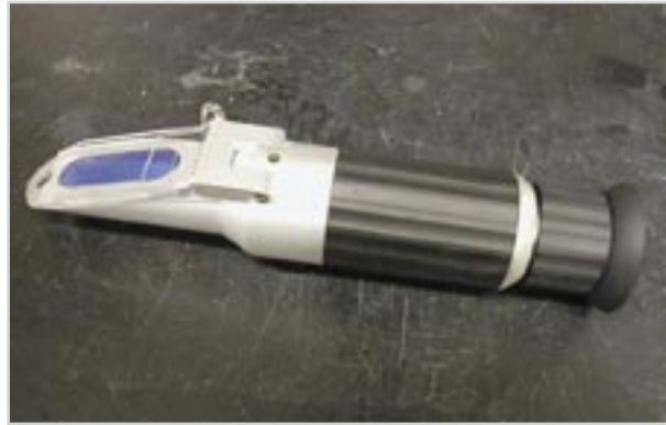
FIGURE 112. A refractometer is used to determine the soluble solids (°Brix) content.
