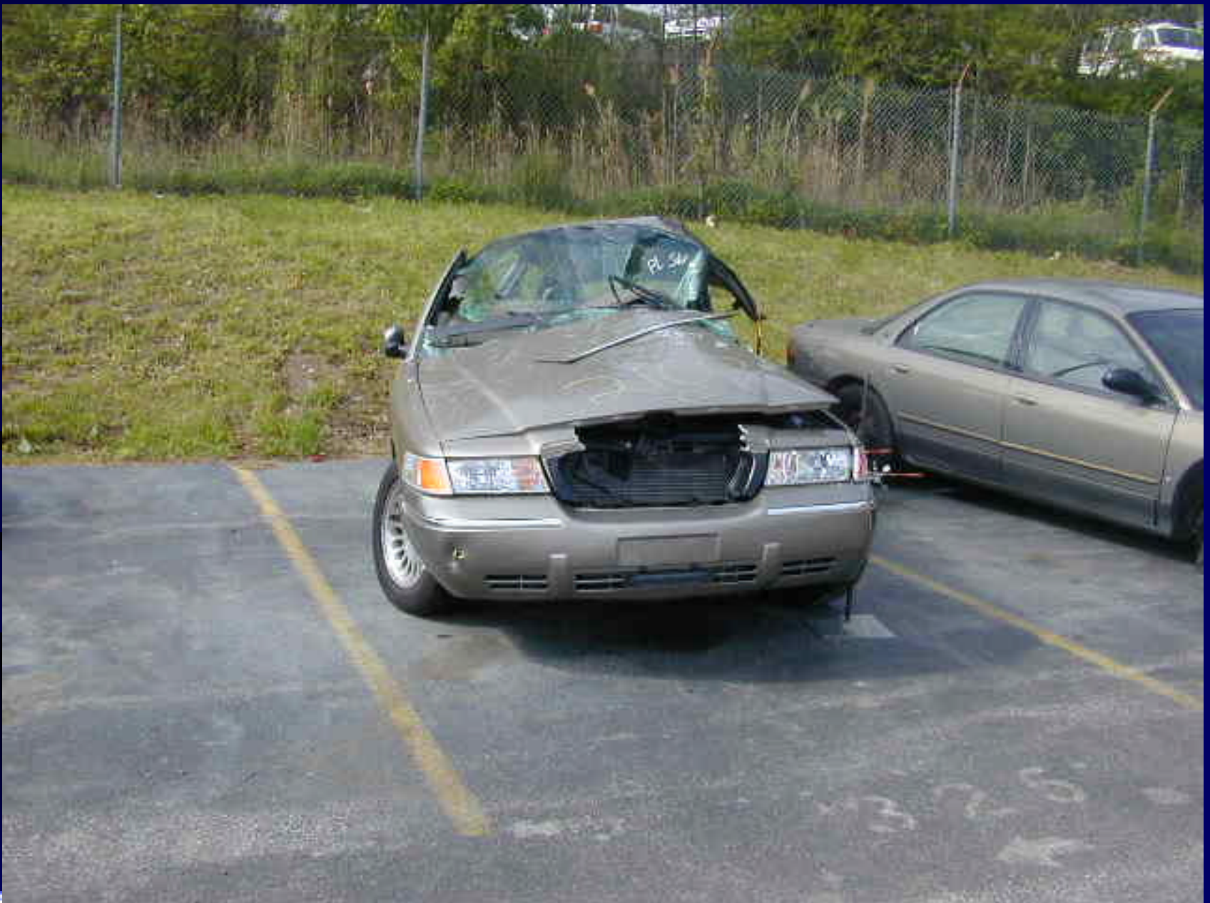
Frontal Damage to Case Vehicle
