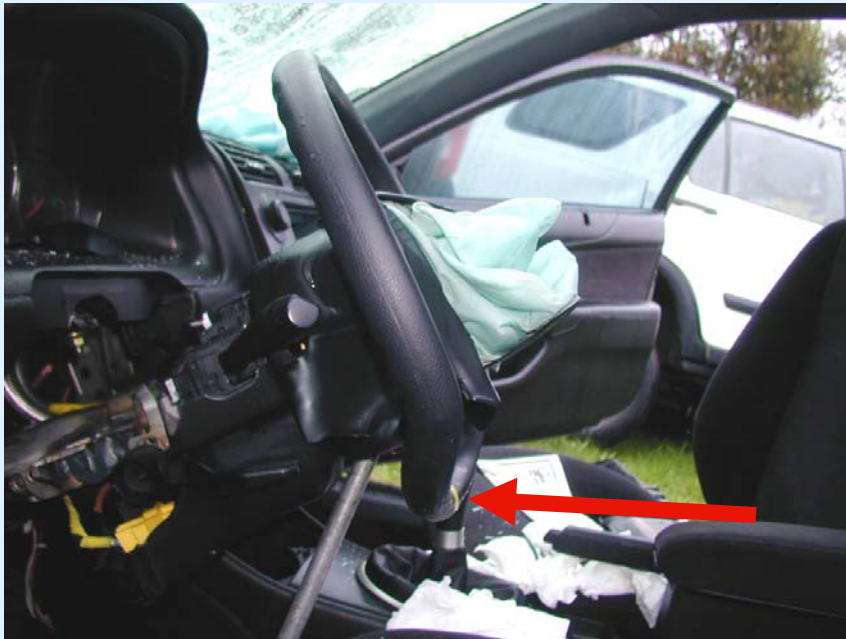
Steering Rim Deformation
