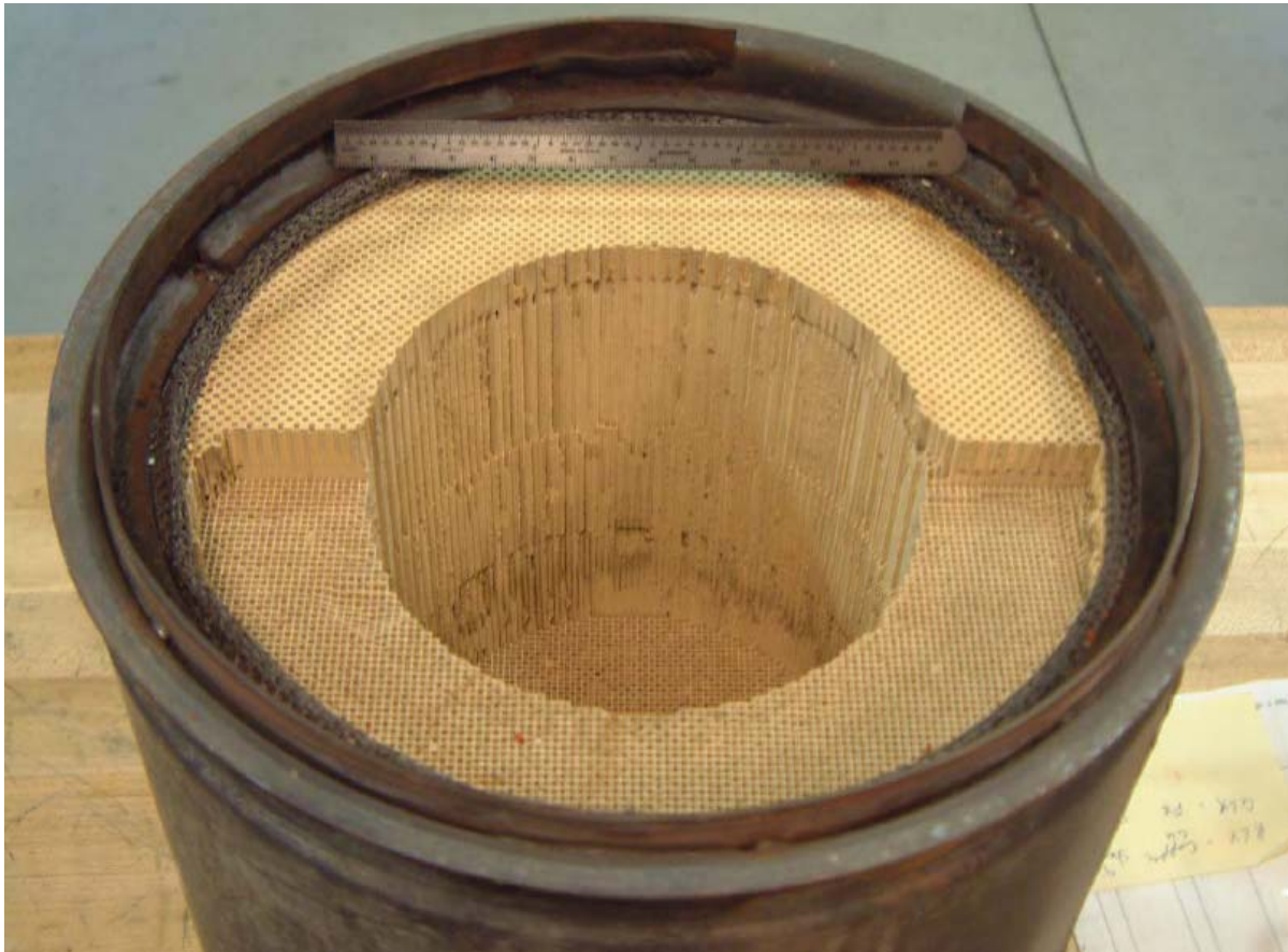
Figure 5. Rear Face of DPF Modified to Simulate Missing Substrate Due to Melting During Un-Controlled Regeneration
