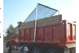
What to do: Top: a tarping station Bottom: an automatic tarper
