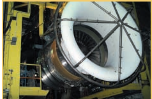
PW4000 low-nitrogen-oxide engine combustor test.
