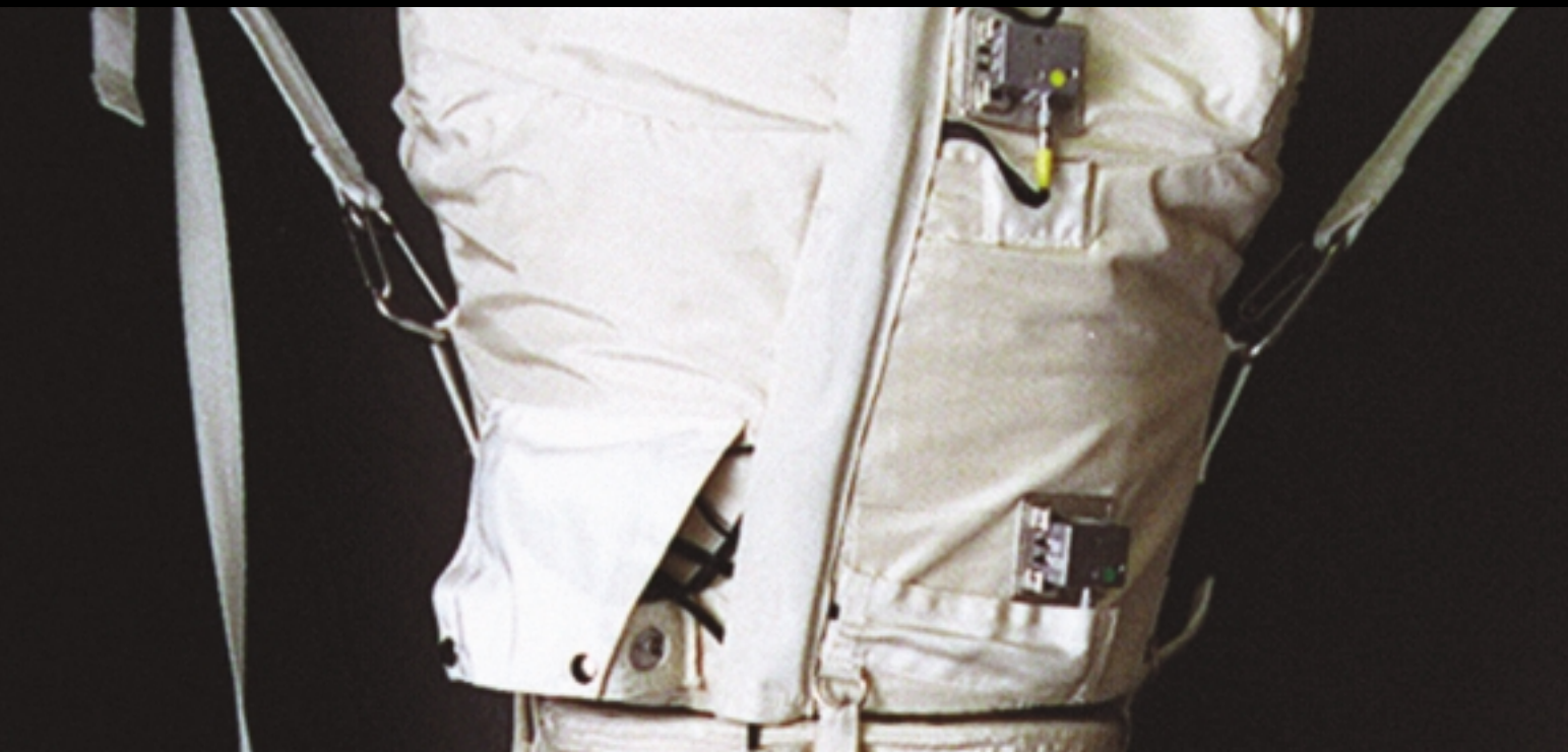
Figure 20: Torso Model with Radiation Measuring Devices
