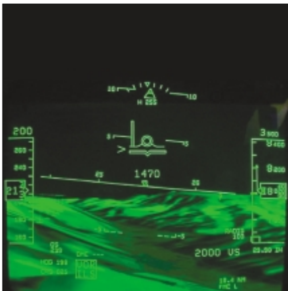
Figure 32: Synthetic Vision Display
