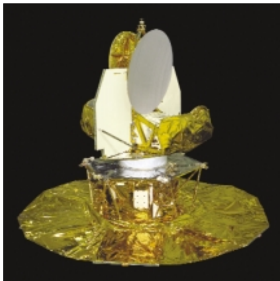
Figure 9: Microwave Anisotropy Probe (MAP) Spacecraft
