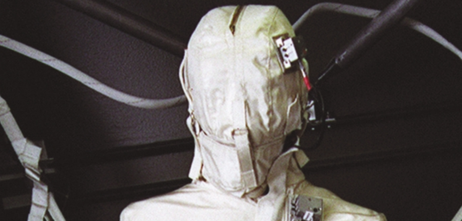
Figure 20: Torso Model with Radiation Measuring Devices
