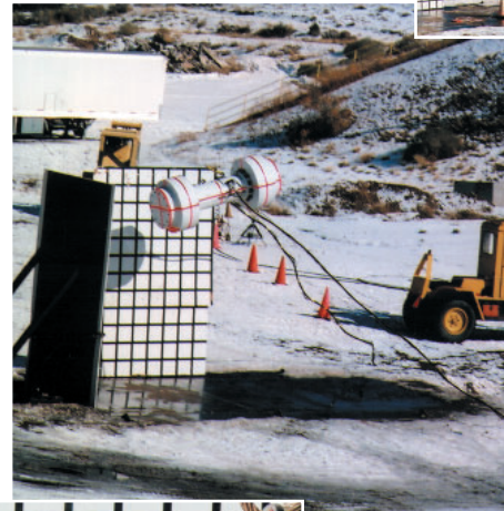
A scale-model container "drop test" helps researchers understand the forces involved in typical and unusual crash situations.
