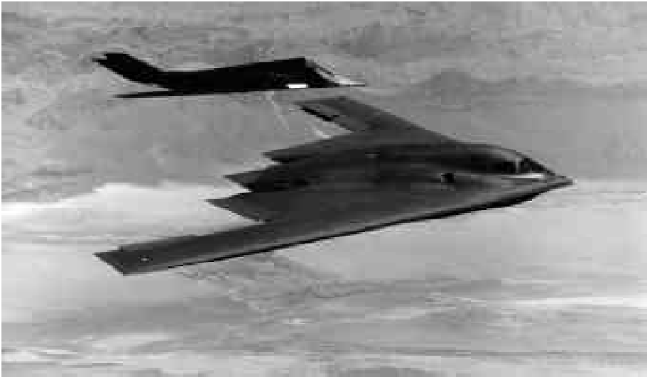
Dissimilar stealth technologies characterize the F-117A and the B-2, but fly-by-wire is needed by both. (U.S. Air Force photo).
