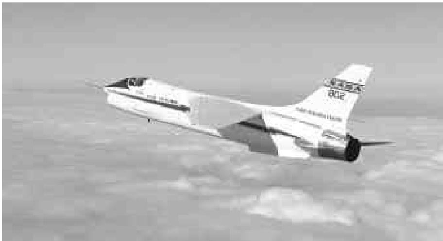
The digital fly-by-wire aircraft caught above a rare cloud layer. (NASA photo ECN-3276).
