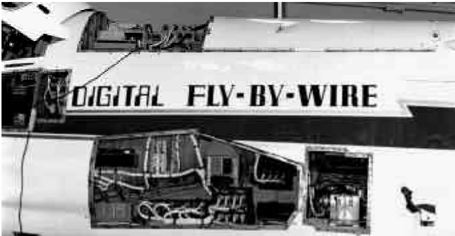
The Apollo hardware jammed into the F-8. The computer is partially visible in the avionics bay at the top of the fuselage behind the cockpit. Note the DSKY in the gun bay. (NASA photo E-24741).
