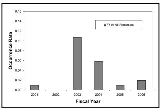
**Figure 5.** Precursors involving LOOP events occurrence rate by fiscal year. No trend line is shown because no statistically significant trend (p-value = 0.85) is detected for the FY 2000–2006 period.
