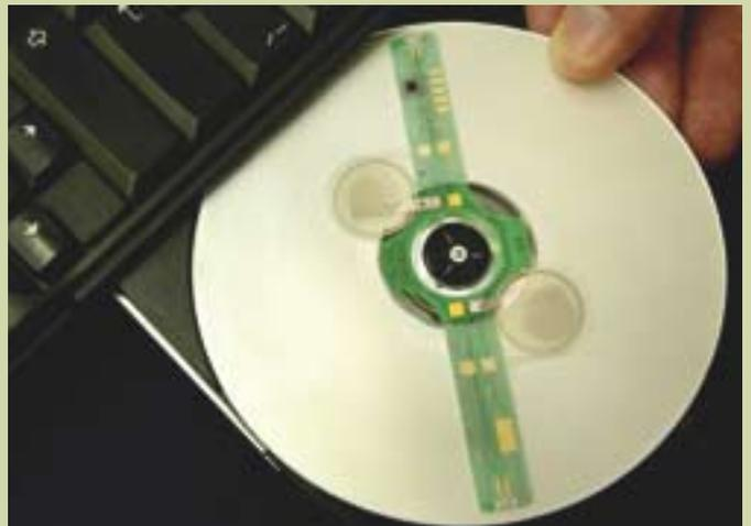
An inventor in Israel, Amos Loewidt, believes he has found a solution to the worldwide problem of CD piracy by placing a slender, plastic-covered electronic card with an electronic chip, a unique serial number, and two optical detectors onto a CD.
