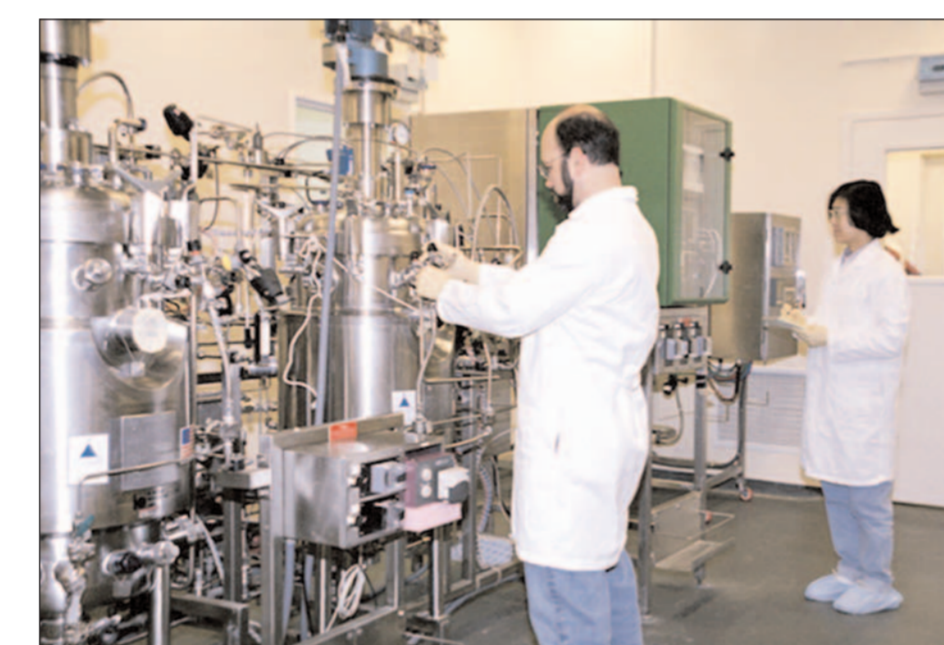
GMP fermentations can be performed at a 20 or 1,000 liter scale.
