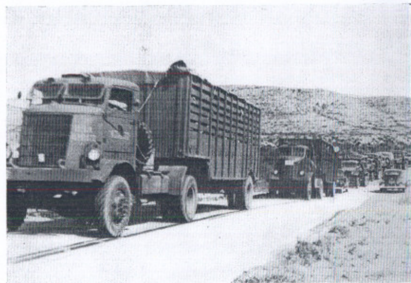
Military convoys would not unduly interfere with passenger and commercial traffic if the highways were adequate in pavement and shoulder width. This Army truck train in Texas completely occupied the lane in its direction of travel, and forced opposing vehicles part way off the road.
