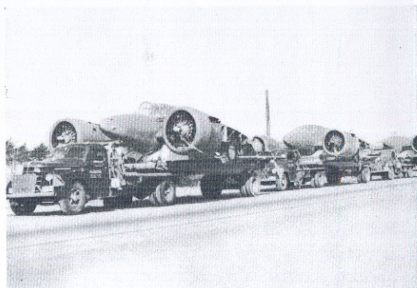
During World War II the motortruck was part of the production line, often extending across many States. These airplane fuselages were hauled from Michigan to Texas for final assembly.
