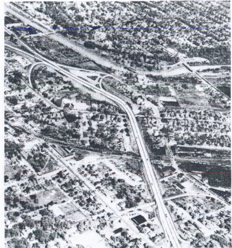
Elimination of main-line railroad grade crossings in urban areas often requires extensive construction, as is evident in this sketch of a proposed treatment on U S Route 40 in Ohio.
