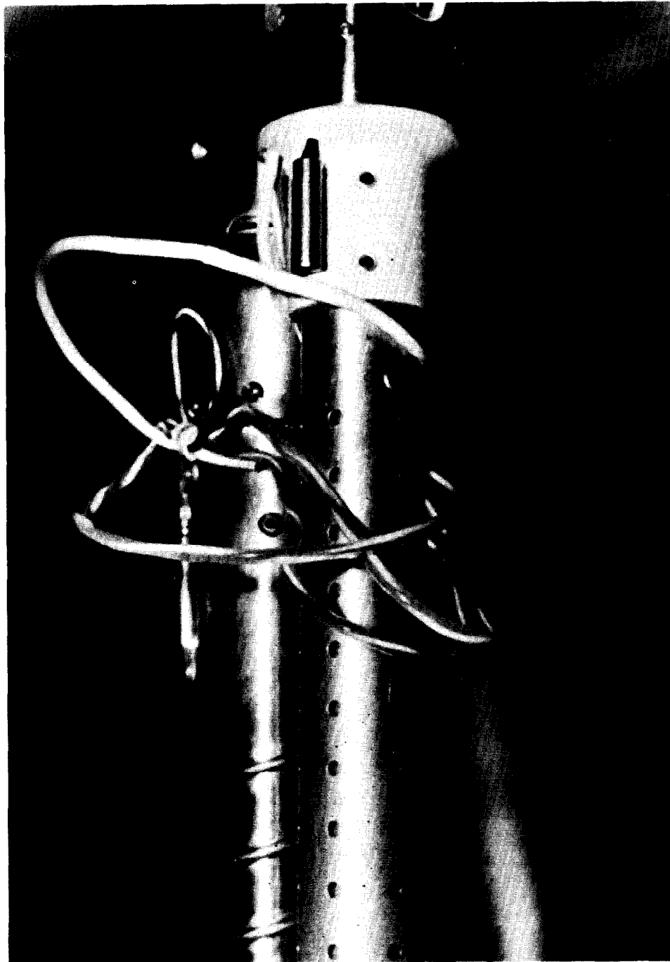
Figure C-4.45 - View inside of tank of typical wire routing from heater probe to quantity probe.
