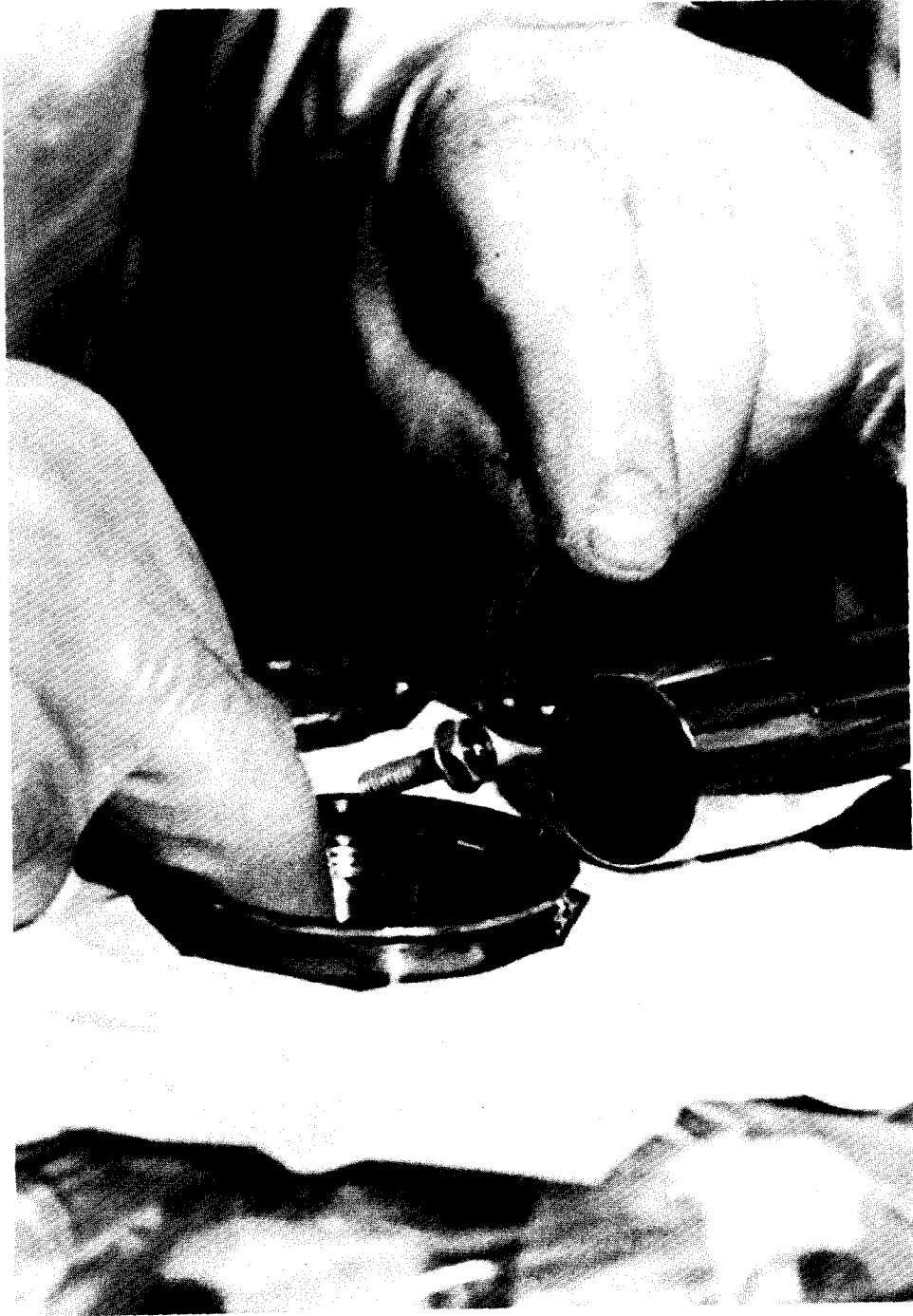
Figure C4-35.- Wire loop used to install heater probe retaining bolt.
