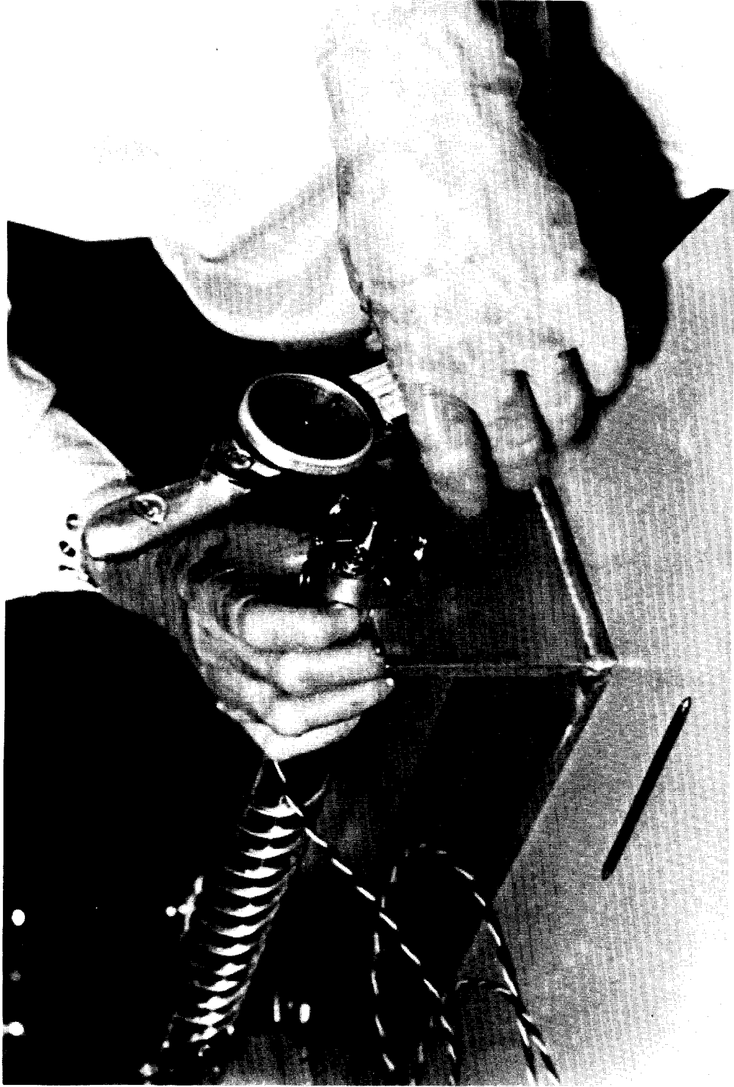
Figure C4-11.- Tightening the motor end cap bolts to establish the proper torque.
