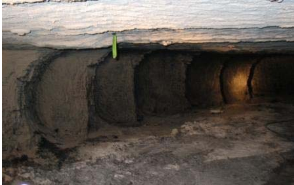
Figure 4.3 Rugged rib condition created by the local mining practice.
