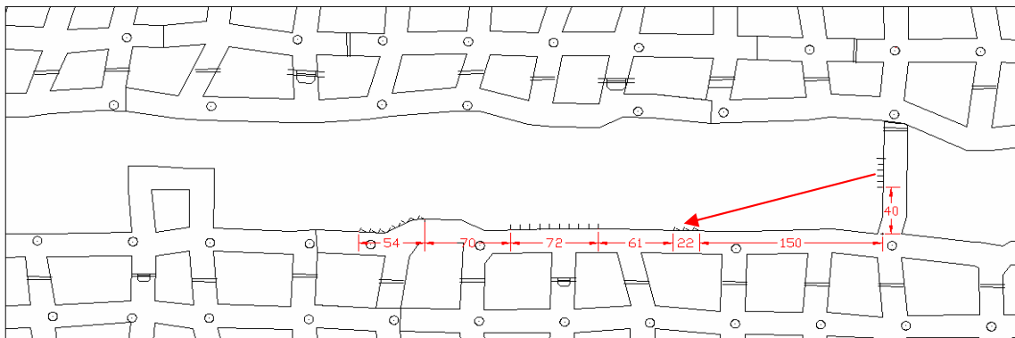
Figure 4.8 Ray paths associated with the transmission survey at Black King.
