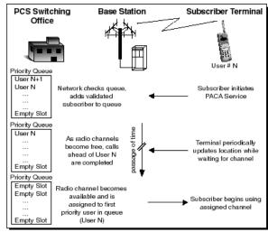
Figure 3. Priority Treatment for NS/EP Telecommunications in a Personal Communications Environment
