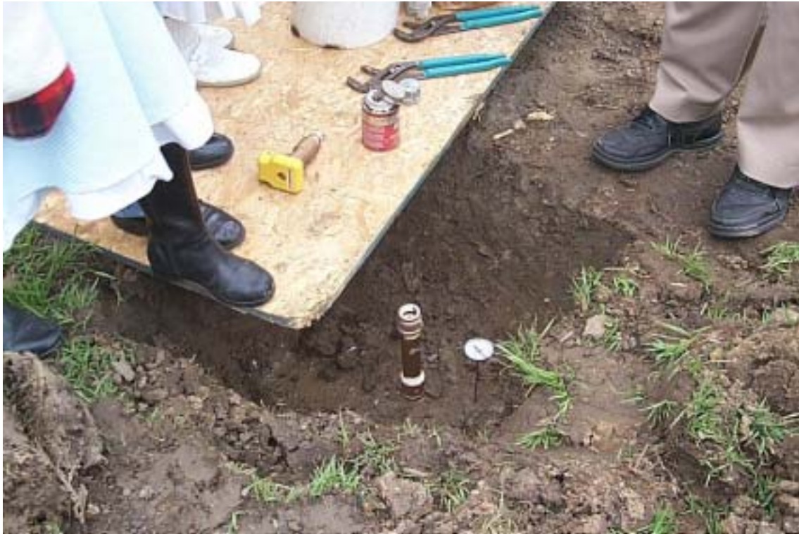
Figure 3.3 Soil Temperature Check
