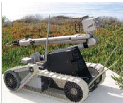
Deployer module mounted on iRobot packbot
