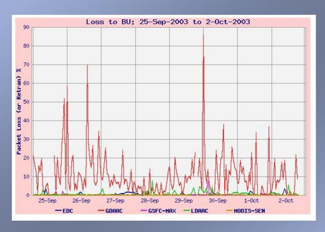
On the other hand, this **Packet-Loss** chart shows low packet-loss to BU from most of the source nodes, but high losses from one source. This would indicate a problem closer to the source node.
