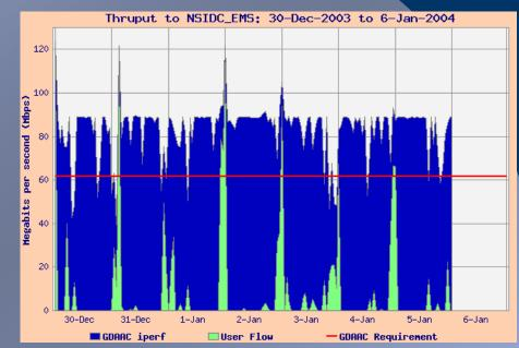
The thruput chart (on the left) shows deep periodic iperf drops (red line), while the integrated chart shows that these low iperf results correspond to high user flows.
