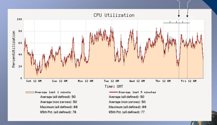
For a test, NetFlow was turned off from 2/12/04 9:30 AM to 2/12/04 5:00 PM Router: ecs\_gsfc, 30 Minutes averages
