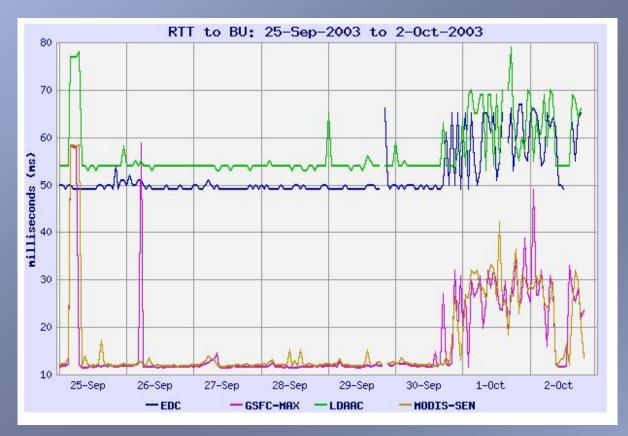
This **Round Trip Time (RTT)** chart shows RTTs between the same hosts and the performance test host at BU. It reveals the benefit of displaying multiple sites on the same chart. In this case, all source-destination pairs experienced significant RTT increase at the same time. This would place the problem closer to the BU end.
