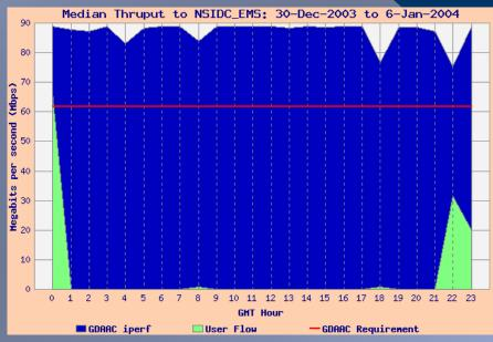
The thruput chart (on the left) shows that iperf drops for 3 hours around midnight (red line), while the integrated chart shows that these hours correspond closely to high user flows.
