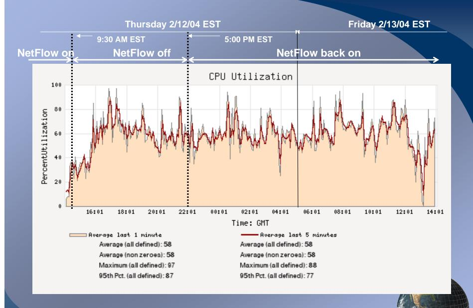
For a test, NetFlow was turned off from 2/12/04 9:30 AM to 2/12/04 5:00 PM Router: ecs\_gsfc 5 minute averages
