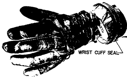
FIGURE 5-27.—Pressure-suit gloves showing cuff slip joint.
