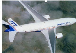
21% thicker faster wing than 757, 767 technology
