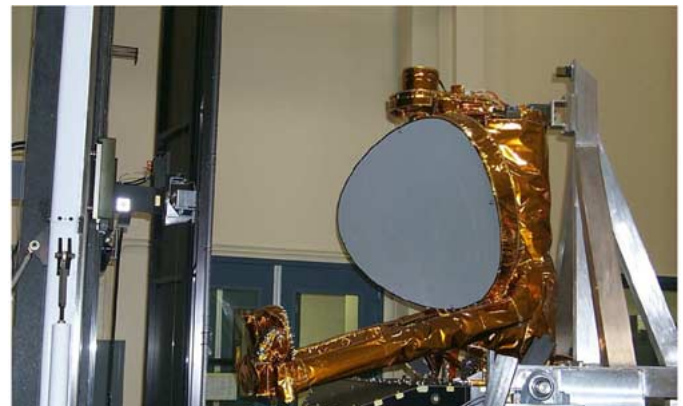
Fig. 7. GHz Module in the Near-Field Range for definitive FOV calibration after environmental tests. The camera was near theodolite station 2 in Fig. 6.
