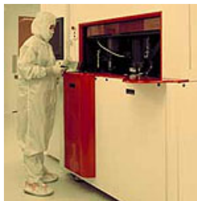
Figure B.9. An SFIL machine (courtesy of Molecular Imprints, Inc.).
