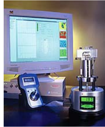
Figure B.16. An AFM configuration (courtesy of Veeco Metrology).
