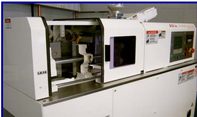
Figure 2.6. High-rate processes such as injection molding can be adapted to manufacture parts with nanoscale features at seconds per part. The questions include how the polymer will flow in nanoscale channels and pits (courtesy of C. Barry and J. Mead, University of Massachusetts, Lowell).
