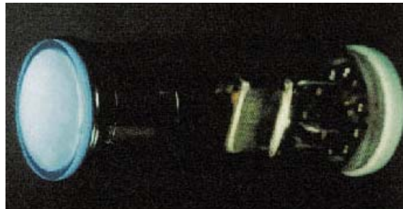
Figure B.21. A nanotube-based jumbotron lamp (© 2000 Elsevier; reprinted by permission from [7]).
