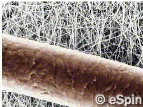
Figure 2.2. A human hair in a nanofiber background. Random mats for filtration and scaffolds are commercially available, but more ordered nanofiber structures are not yet manufacturable (courtesy of eSpin Technologies).
