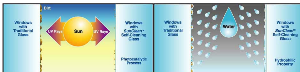
Figure B.10. Photocatalytic and hydrophilic processes in self-cleaning of glass (courtesy of PPG).
