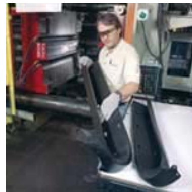
Figure B.2. Nanocomposite step-assist for vans (courtesy of GM/Blackhawk Automotive Plastics).
