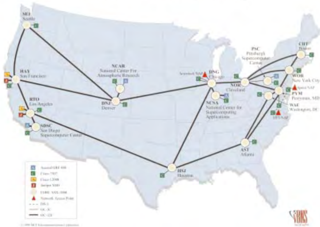
The very high performance Backbone Network Service (vBNS) backbone network service that provides high performance connectivity among NSF research sites and Internet2 gigapops.
