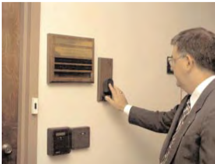
NSA's Technology Demonstration Center provides a showcase for many of the agency's most innovative developments. Access to the facility is controlled by a customized fingerprint recognition system, pictured at the left.
