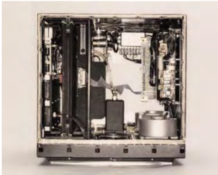
Pictured is the diamond Multi-Chip Module (MCM) aerosol spray cooled Cray J90 supercomputer mounted vertically in the black “clamshell enclosure” on the left. One redundant aerosol spray pump/heat exchanger is visible as a silver cylinder on the lower right. The pump controller-fail safe electronics are visible in the upper right. Mounted on the far left wall of the integration platform are the internal power supplies for the pump control electronics.
