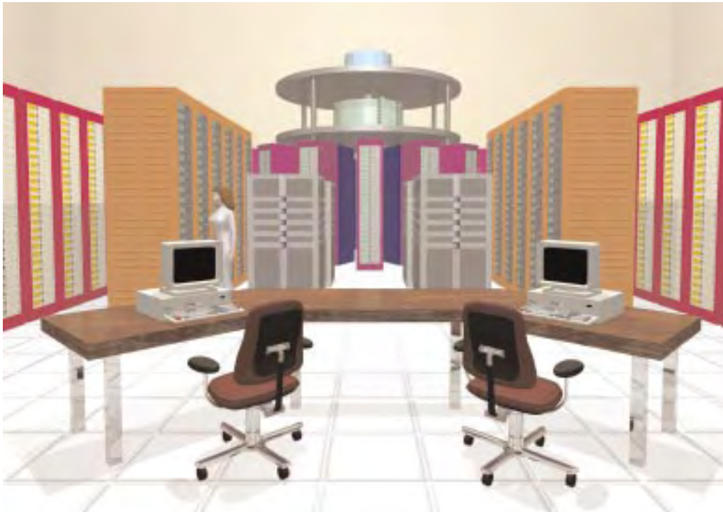
Artist's 3-D depiction of a prototype computing system employing HTMT architecture. DARPA, NASA, and NSA researchers are evaluating the feasibility of constructing a hybrid HTMT system that would be capable of a sustained rate of 10^5 floating point operations per second (one petaflop).
