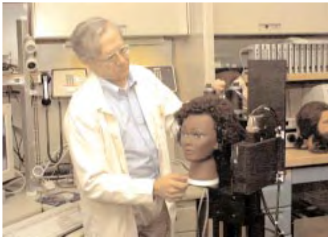
Face recognition can provide instant hands-free access control to computer workstations. Pictured above left and right are two views of an experimental 3-D face recognition system being tested at NSA. The system uses infrared imaging techniques. Pictured left is an NSA researcher preparing to test the face recognition system using a computer-controlled precision positioning platform.
