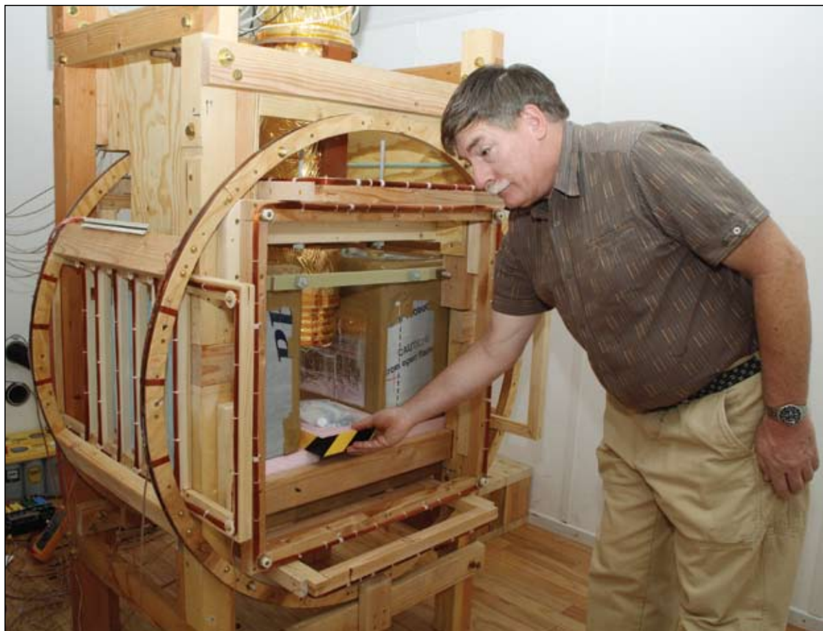
James Sims of Applied Engineering Technology-1 loads a sample “3-1-1” baggie into the ultra-low-field magnetic resonance system. The system, created by the “SQUID” team in Applied Modern Physics for brain imaging applications, is now being developed for screening carry-on liquids at airports. The work is a collaboration between the “SQUID” team and engineers from the Applied Engineering and Technology; Accelerator Operations and Technology; Information Resource Management; and International, Space and Response divisions. Photo by Sandra Valdez, Records Management/Media Services and Operations
