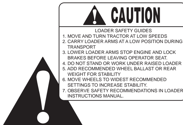
Figure 1. Typical safety sign for front-end loaders.
