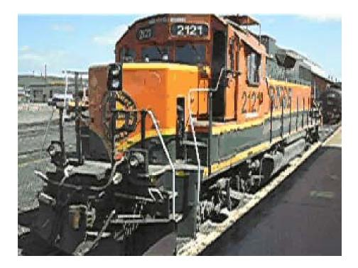
A GP38-2 locomotive consumes 4.5 gallons per hour of fuel at normal idle. When outside temperatures drop to 10-15F, the locomotive is idled at notch 3 to keep the engine warm. At notch 3 the locomotive consumes 11 gph.
