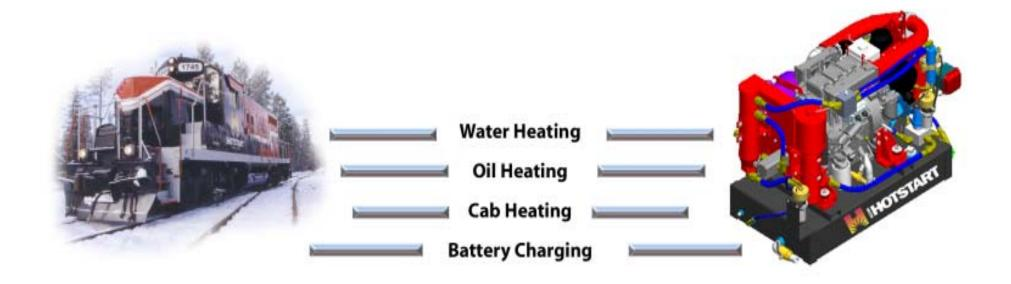
Kim Hotstart's DDHS (Diesel Driven Heating System) was developed in response to the railroads who wanted the flexibility to shutdown their locomotives anywhere and still be able to easily restart the engine when needed.
