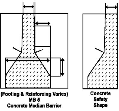
Continuously poured, reinforced, sloped faced, concrete section. Barrier can be anchored by dowels or an asphalt key.
