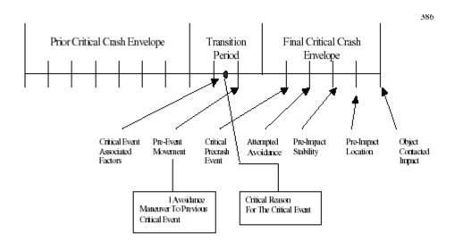
Figure 5 Vehicle's Critical Crash Envelope
