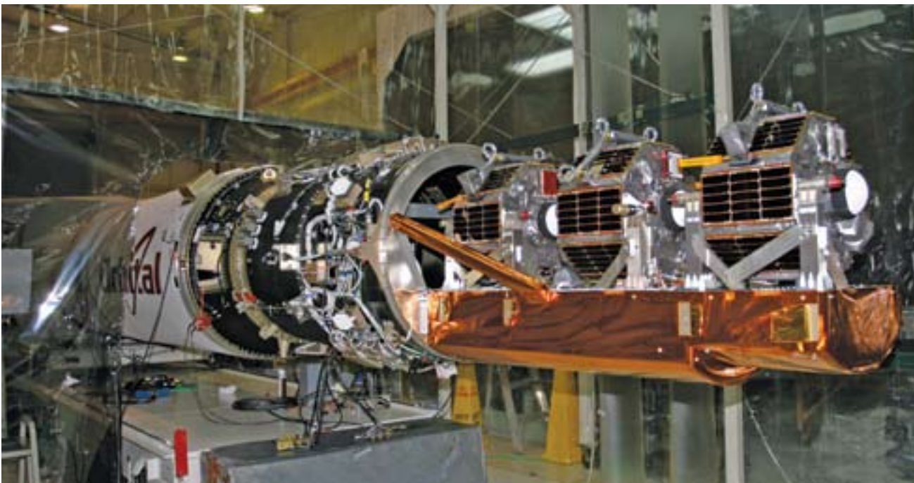
Caption: ST5 spacecraft in Pegasus rocket prior to fairing installation.
