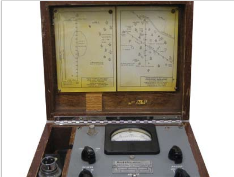
4.26 Soil moisture measuring equipment manufactured by the Beckman Instruments Company. Note the map of the snow course on the inside of the case lid.
