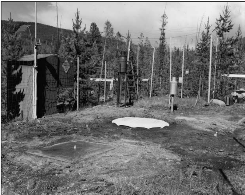
4.32 Testing metal and butyl snow pillows at Lick Creek, south of Bozeman, Montana
