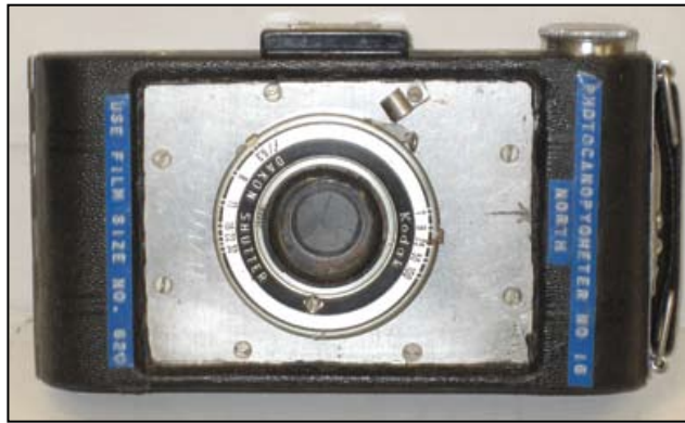
4.38 Kodak camera modified to photograph tree canopies
