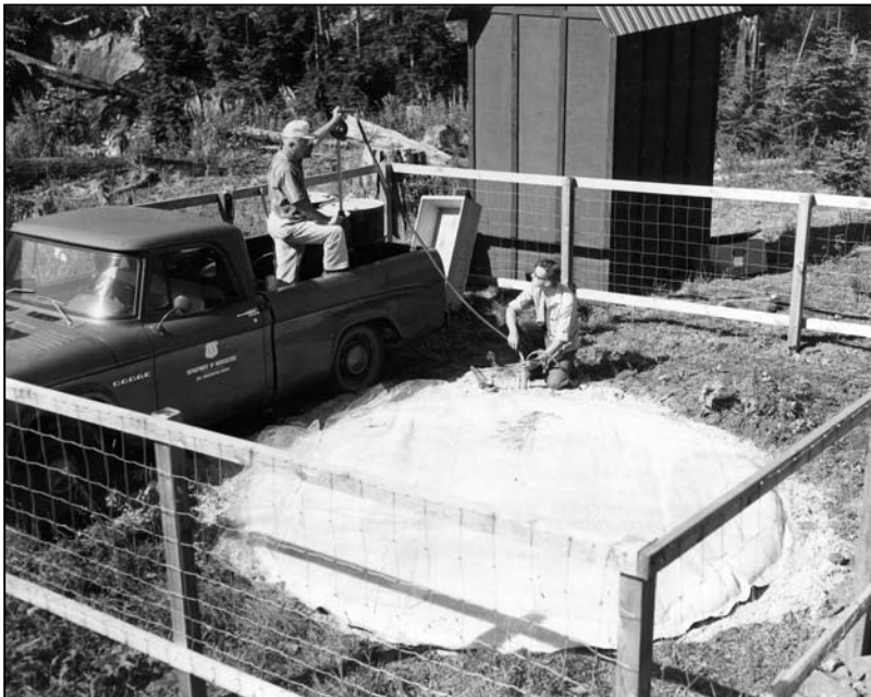
4.13 Installing snow pillow and instrument shelter at Mill Creek Watershed, Washington
