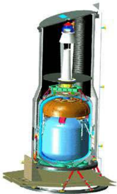
This cutaway drawing shows SIRTf's cryostat, with its helium tank, and the telescope mounted above.
